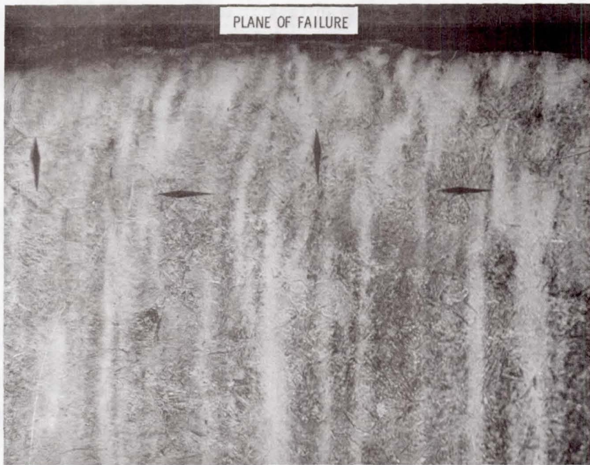
Figure 3. - Banded microstructure at 100X of failed shaft showing failure surface and tukon hardness indentations.
