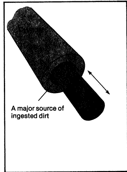
3. Ingested dirt is a major source of contamination, such as at rod seals
