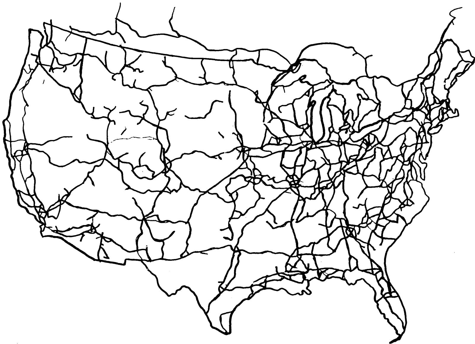
Figure 5-1. Existing Microwave Links (4 and 6 GHz)
