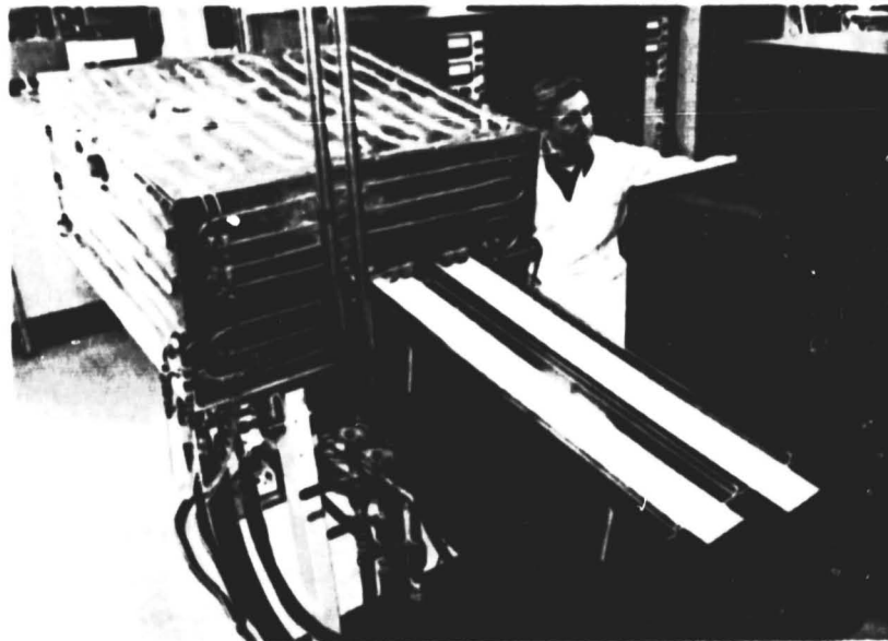
Figure 18. SCIM-II exterior showing two side-by-side substrates entering the coater.
