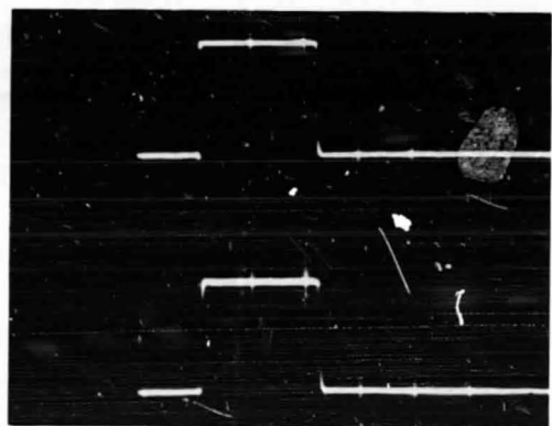
Fig. 6. Scope trace of stable switching pulses. The sample is the same as in Fig.5 with voltage (upper trace) of 2V/div; current (lower trace) of 40 μA/div; time of 5 μsec/div; pulse repetition rate of 10 KPPS; and temp of 345° ± 2°C.
