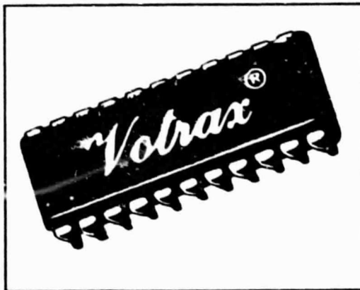
Figure 1. Votrax ® SC-01 Speech Synthesizer
