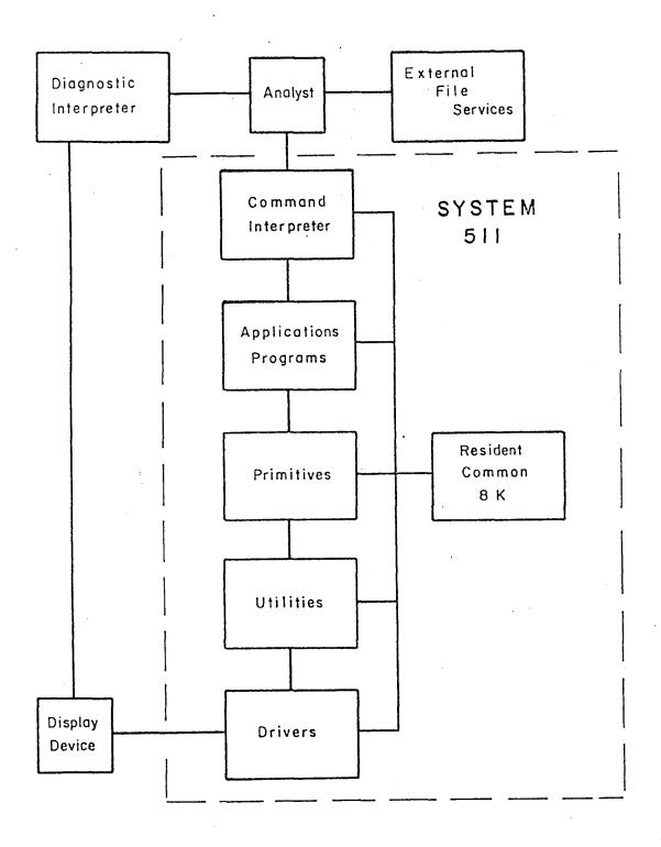
Figure 1 System 511 Software Hieracy Implemented by IDWR On Digital PDP 11/24
