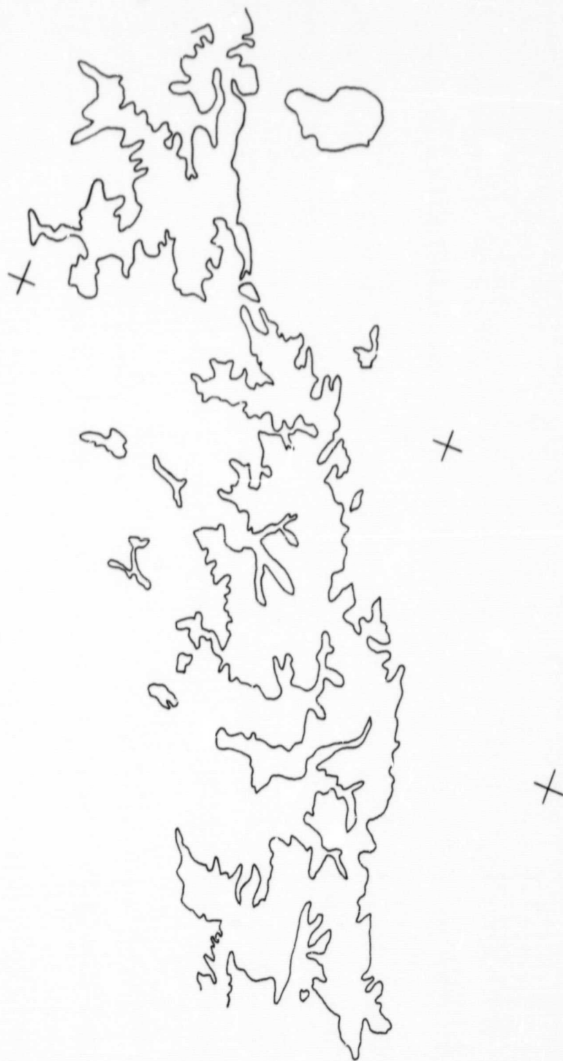
Figure 7-11b Map showing snow line mapped from 20 July Landsat-2 image. Note that although finer detail is apparent in the Landsat image, the overall snow boundary corresponds closely to the snow extent mapped from the HCMM image (Figure 7-10a).
