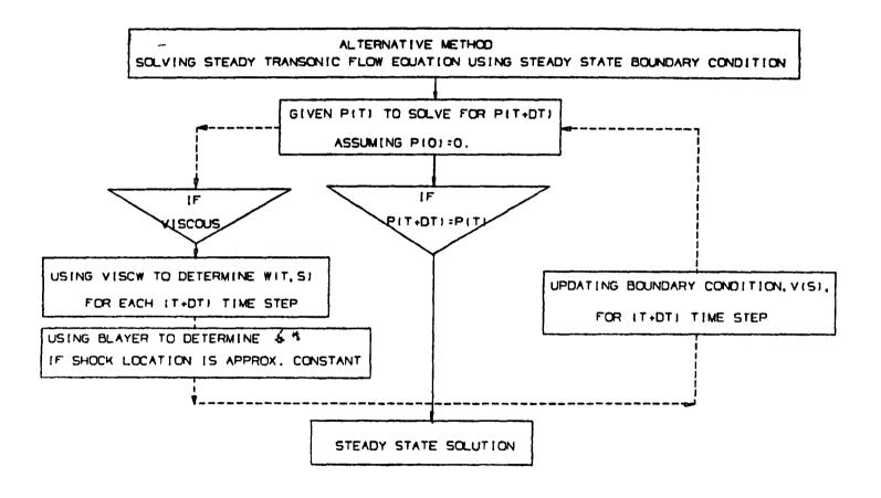
FIGURE IC, FLOW CHART FOR THE ALTERNATIVE METHOD TO OBTAIN STEADY STATE SOLUTION
