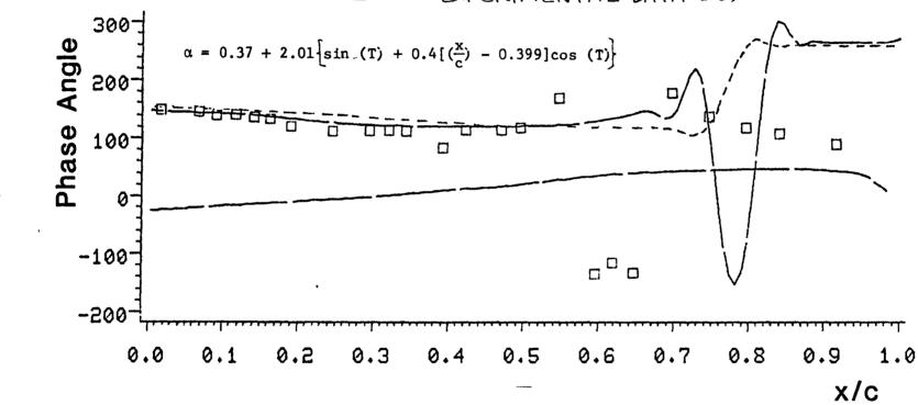
NCR 7301 AIRFOIL MINF=0.752 ALF=0.37 INTEGRATED RESULTS CYCLES 4-5 PITCHING 2.01 DEG. WITH K=0.4 AT X/C=0.399 USING AF2 FOR STEADY SOLUTION
