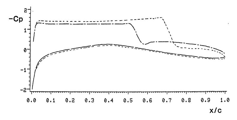
RAE 2822 AIRFOIL MINF=0.730 ALF=3.19 UNSTEADY STATE T=48.12, ALF=2.35DEG. OSCILLATING 1.0 DEG. WITH K=0.2 AT X/C=0.5 UNSTEADY PROCEDURE FOR STEADY SOLUTION
