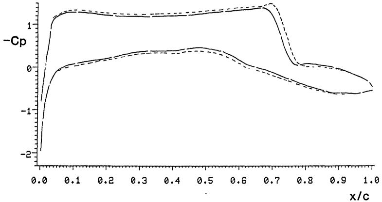
NER 7301 AIRFOIL MINF=0.752 ALF=0.37 UNSTEADY STATE, T=21.12, ALF=1.95 DEG. PITCHING 2.01 DEG. WITH K=0.4 AT X/C=0.399 USING AF2 FOR STEADY SOLUTION
