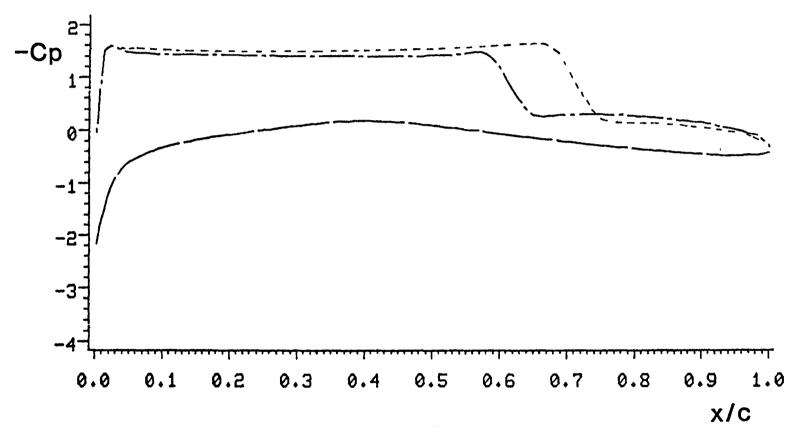
RAE 2822 AIRFOIL MINF=0.730 ALF=3.19 UNSTEADY STATE T=39.41, ALF=4.18DEG. OSCILLATING 1.0 DEG. WITH K=0.2 AT X/C=0.5 UNSTEADY PROCEDURE FOR STEADY SOLUTION
