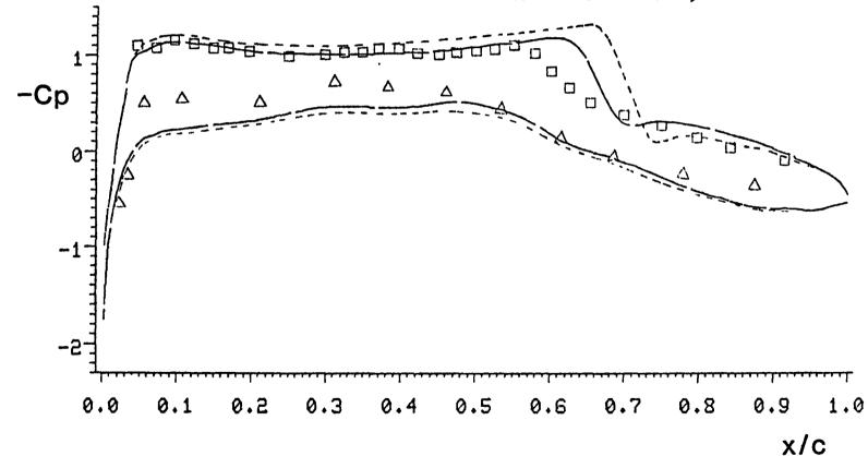
NLR 7301 AIRFOIL MINF=0.752 ALF=0.37 UNSTEADY STATE, T=0.0, ALF=0.37DEG. PITCHING 2.01 DEG. WITH K=0.4 AT X/C=0.399 USING AF2 FOR STEADY SOLUTION
