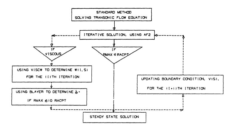
FIGURE IB. FLOW CHART FOR THE STANDARD METHOD TO OBTAIN STEADY STATE SOLUTION
