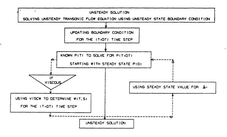
FIGURE ID. FLOW CHART FOR OBTAINING UNSTEADY SOLUTION
