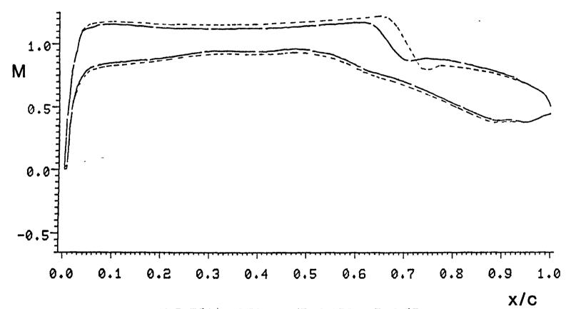
NLR 7301 AIRFOIL MINF=0.752 ALF=0.37 UNSTEADY STATE, T=0.0, ALF=0.37DEG. OSCILLIATING 2.01 DEG. WITH K=0.4 AT X/C=0.399 USING AF2 FOR STEADY SOLUTION
