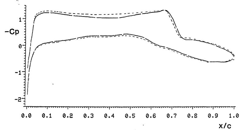
NLR 7301 AIRFOIL MINF=0.752 ALF=0.37 UNSTEADY STATE, T=26.35, ALF=2.43 DEG. PITCHING 2.01 DEG. WITH K=0.4 AT X/C=0.399 USING AF2 FOR STEADY SOLUTION Figure 12, Pressure Coefficient (T = 26.35)
