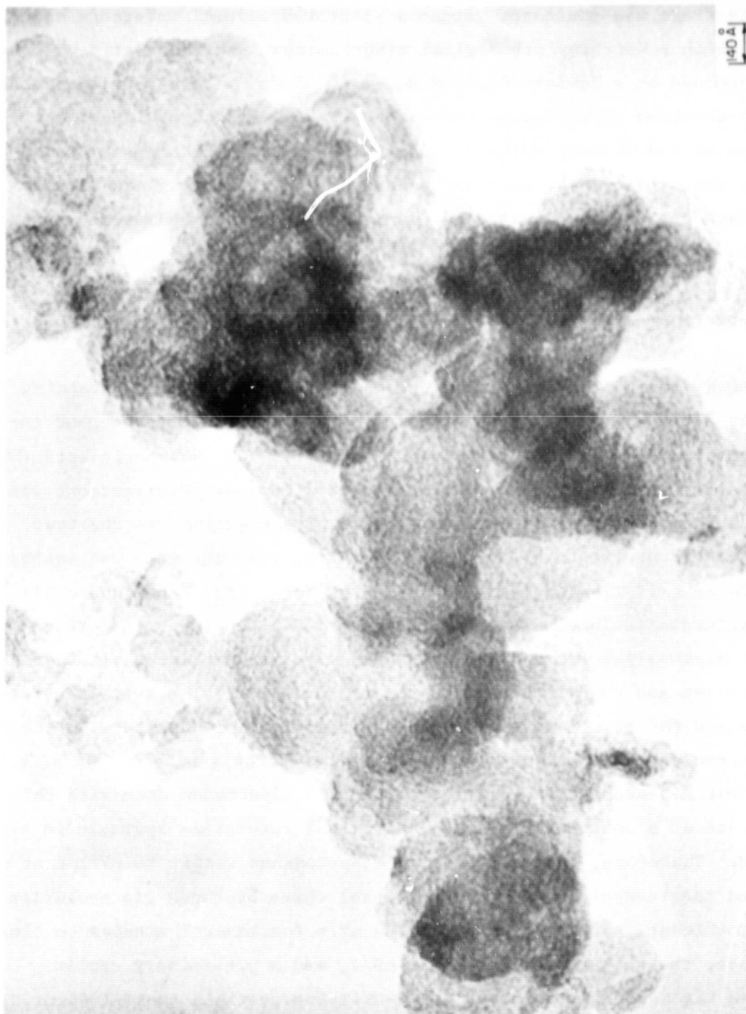
Figure 11. ELECTRON MICROGRAPH OF 5% PLATINUM ON SUPPORT VFEn-15
