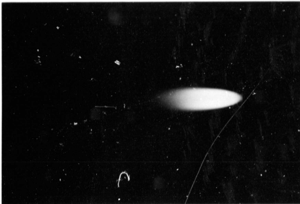
Figure 3-5: Photograph of the combustor in operation under 30^\circ counter-swirl, propane firing.
