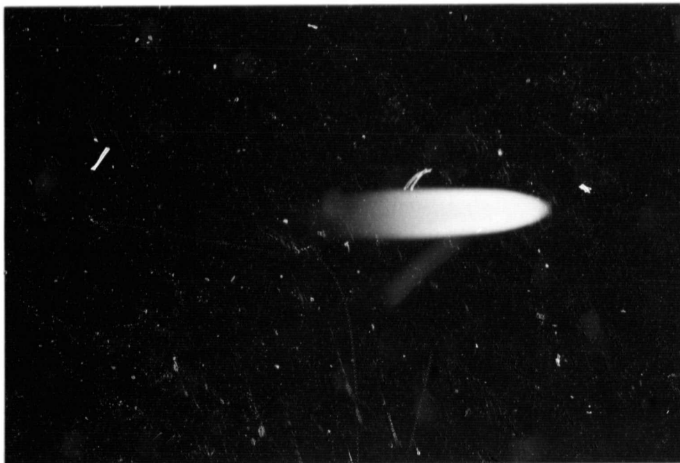
Figure 3-4: Photograph of the combustor in operation under 30^{\circ} co-swirl, propane firing.
