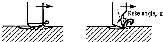
(b) Deformation and fracture due to a cutting tool.
