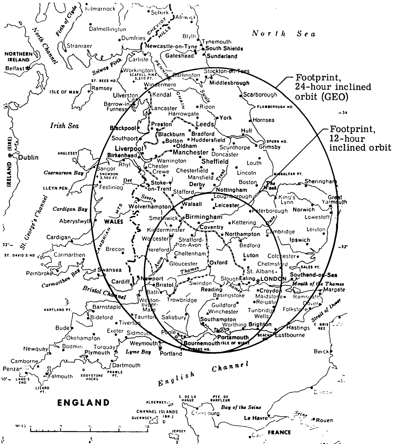
Figure 7.- Illumination of England from 12- and 24-hour orbits.
