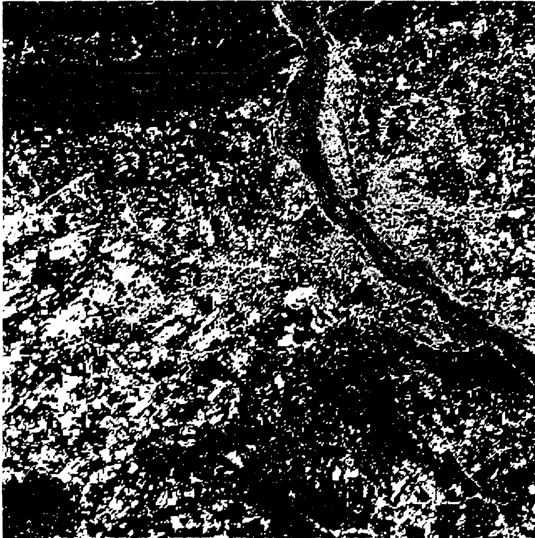
Figure 5-28. Printer/plotter map of density levels in IDIMS display of Landsat band 5, Harrisburg subscene.
