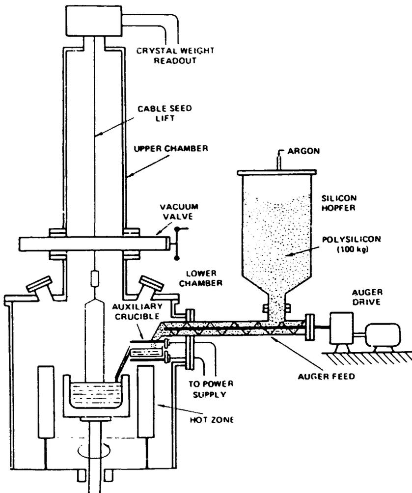
IN THE T.I. SYSTEM, THE AUGER FEEDER INTRODUCED SILICON INTO A SMALL PREMELTER. THE LIQUID SILICON THEN FLOWED INTO THE CRUCIBLE, THEREBY MAINTAINING A CONSTANT MELT LEVEL DURING GROWTH.
