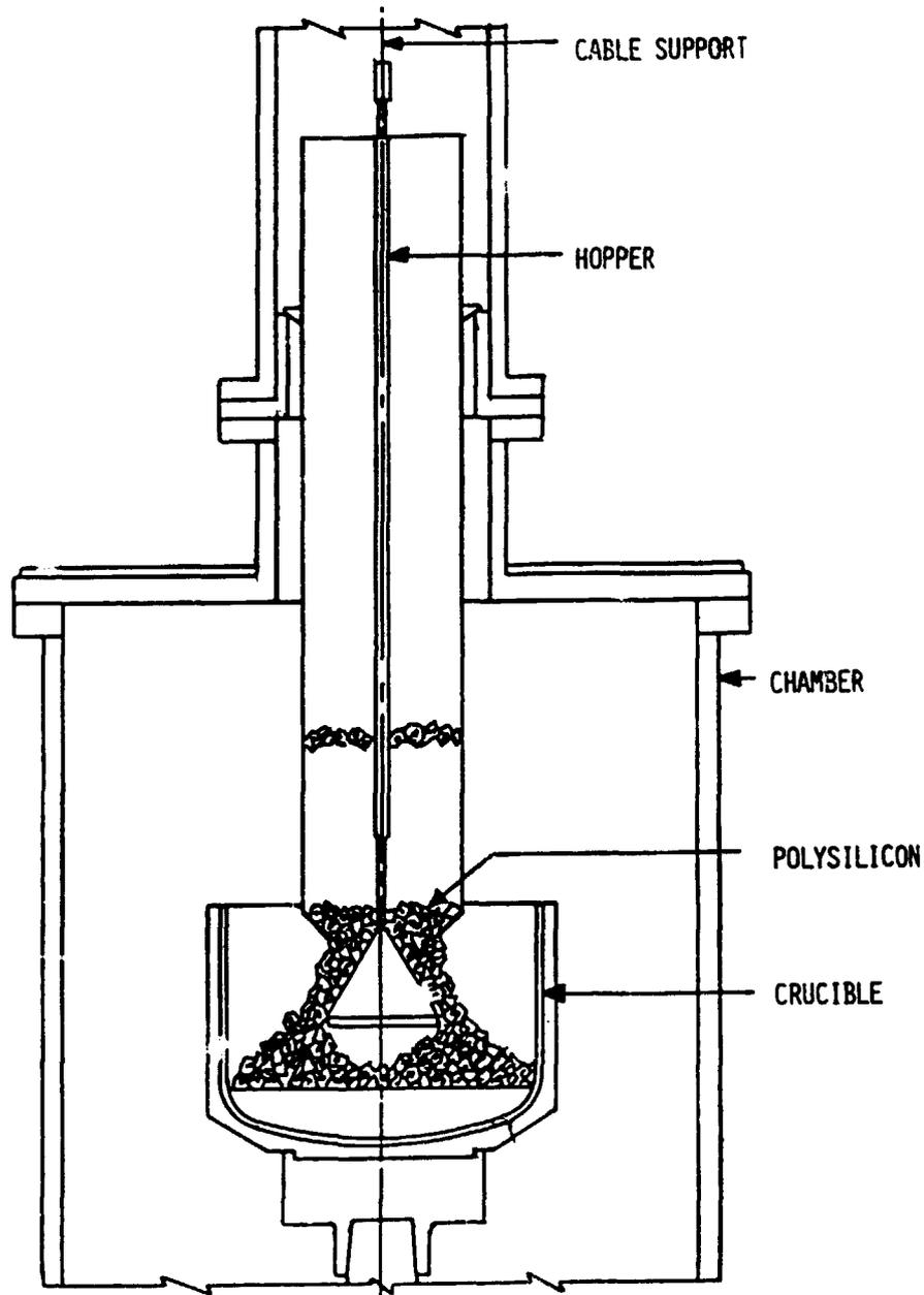
A SELF-DUMPING HOPPER WAS THEREFORE DESIGNED AND BUILT WHICH HAD ABOUT A 16 KILOGRAM CAPACITY. IT WAS A SIMPLE DESIGN AND QUICKLY BECAME THE PREFERRED METHOD. AS THE HOPPER IS LOWERED, IT COMES TO REST ON A RING AT THE ISOLATION VALVE. THE PLUG SUPPORTING THE CHARGE AT THE BOTTOM OF THE HOPPER CONTINUES TO LOWER AS THE SUPPORTING CABLE IS LOWERED, EFFECTING COMPLETE DISCHARGE OF THE SILICON.
