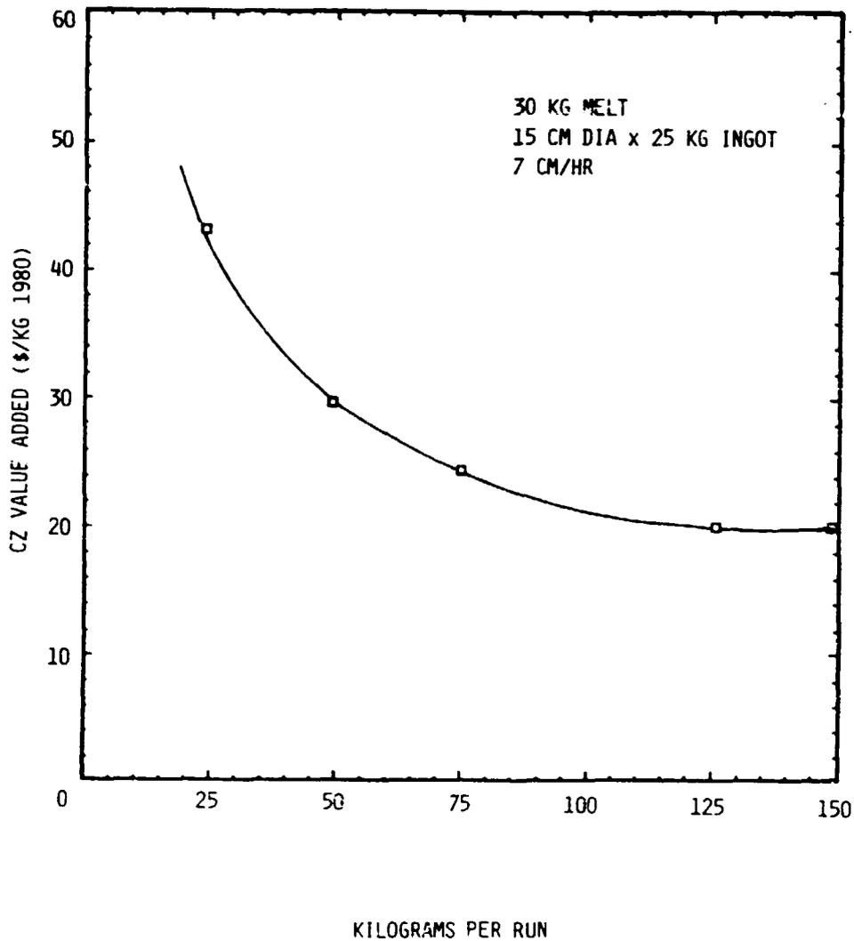
THE SENSITIVITY OF RUN SIZE UP TO 150 KILOGRAMS IS SHOWN IN THIS SLIDE. IT SHOWS A SUBSTANTIAL REDUCTION IN COST BY THE GROWTH OF TWO OR THREE INGOTS FROM ONE CRUCIBLE. THE COST BENEFIT BECOMES MARGINAL IN THE 100-150 KILOGRAM RANGES.
