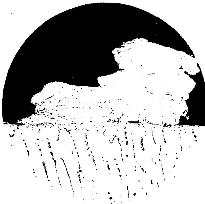
Figure 1.- Severe surface welding resulting from unlubricated sliding (2% Al-Ni alloy from 10 -9 mm Hg vacuum experiment).
