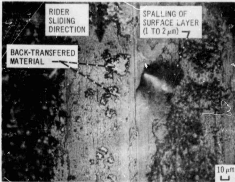
(c) Wear surface on group 111 type polyimide. Figure 5. - Concluded.
