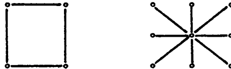
Figure 19. Bi-Cubic Rectangle and Grid Point Stencil
