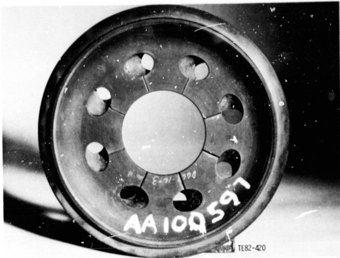
Figure 22. Ceramic combustor swirl plate (dome).
