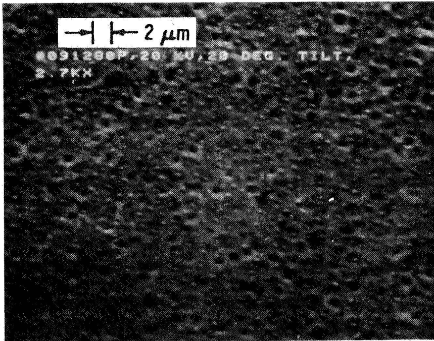
Fig. 1. SEM photomicrograph of a typical Ge film grown at 700°C on a (100) Si substrate, before laser annealing.
