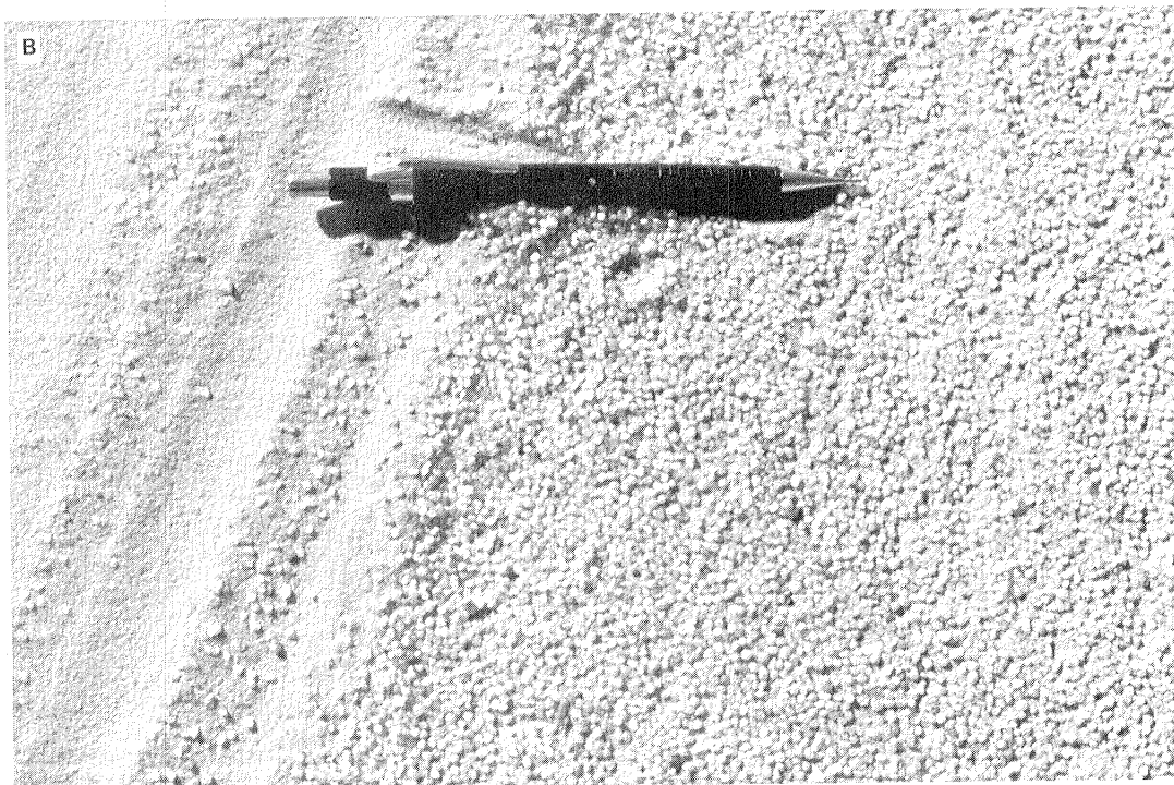
Figure 12.3 (A) Flat surfaced (truncated?) ripples of coarse lag deposits east of the Gilf Kebir. Planar surface may result from high speed winds needed for redistribution of lag. (B) Closely-spaced lag and underlying sand deposits of flat-topped ripples. Mean grain size of lag fraction is -0.75 \phi (1.7 mm). Pencil is 14.5 cm long.
