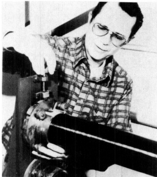
(c) Rotating half-strut for length adjustment.
