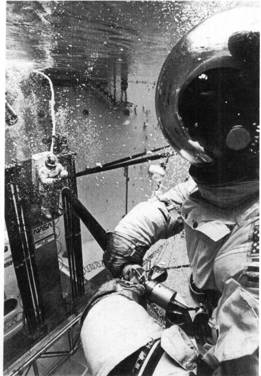
Figure 16.- Installation of strut by two test subjects.
