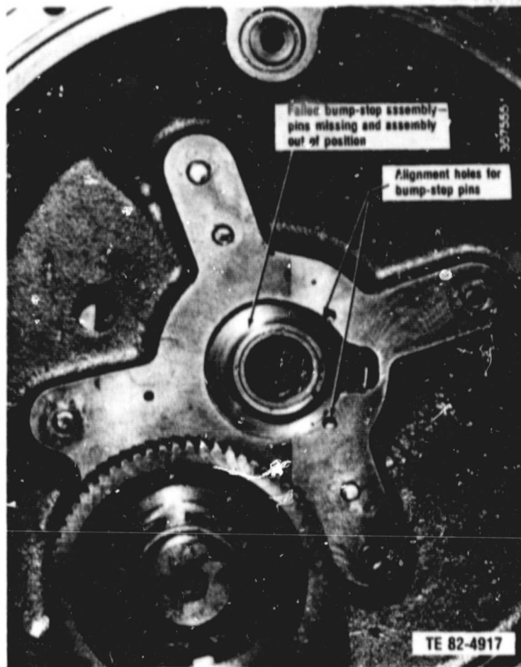
Figure 8. Gearbox front housing from Greyhound engine S/N T5 showing misoriented bump stop and pins missing (508 total engine hours).
