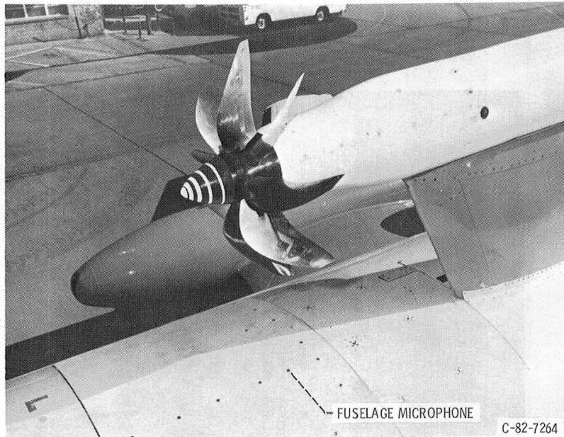
Figure 2. - Advanced-propeller (SR-3) installation on the jetstor.
