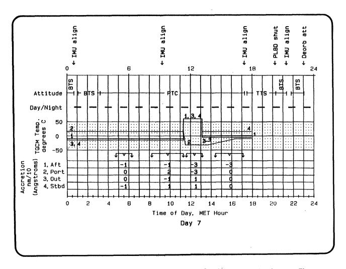
The data shown for day 7 is taken from the real-time transmissions. These are available only when the Orbiter passed over an appropriate ground station.
