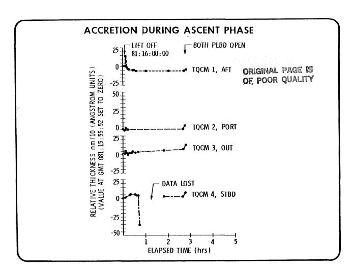
This figure shows the accretion indicated by the four TQCM's during the launch and early orbital phase. Note that the zero value has been set as the values indicated by the TQCM's at about 4 minutes prior to launch. (Launch occurred at 081:16:00:00~GMI.) The TQCM's were set to be controlled at +15°C during these phases.
