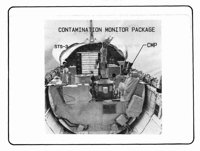
This figure shows a view of the Columbia and many parts of the OSS-1 pallet. The Contamination Monitor Package (CMP) is the small box shown within the circle.
