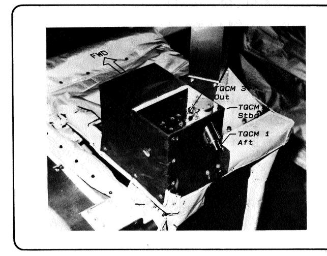
This is a view of the CMP. It is roughly 20 cm high, 18 cm wide, and 30 cm long (8x7x12 inches). It weighs about 7 kg (15 pounds). The average power consumption is about 7 watts. The box itself is passively thermally controlled using silver teflon for radiating surfaces and aluminized kapton multi-layer insulation for radiation isolation.
