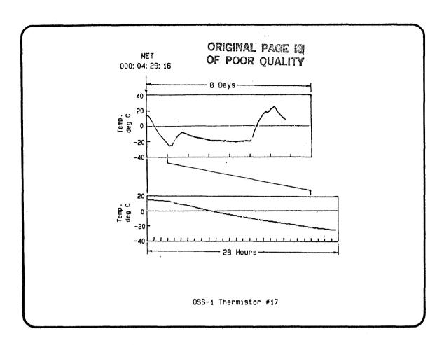
The STS-3 mission involved three major attitudes with respect to the sun for the purpose of verifying the Orbiter thermal design. These were: tail to the sun (TTS) with the orbiter bay always facing away from the earth; nose to the sun (NTS) where the roll rate allowed the orbiter to view the earth, and bay to sun (BTS) where the orbiter bay faced the sun. The TTS condition provided a very cold condition, NTS a moderately cold condition, and BTS a very hot condition.
