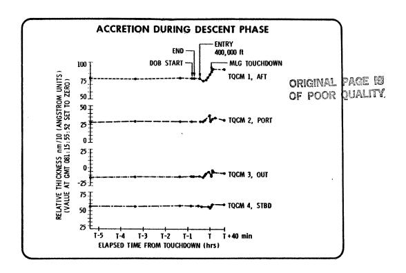
The data on this figure is referenced back to approximately 4 minutes prior to launch. TQCM 1 was set to  $0^{\circ}$ C, TQCM 2 to  $-10^{\circ}$ C, TQCM 3 to  $-5^{\circ}$ C, and TQCM 4 to  $+15^{\circ}$ C in preparation for entry. The system was designed to hold these temperatures through the landing phase.
