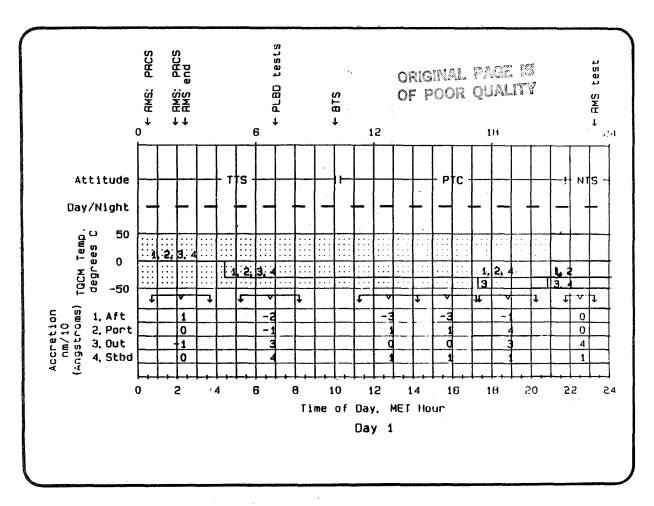
While in the NTS mode, a bake-out of the TQCM's was conducted. This involved raising their temperatures to  $+60^{\circ}$ C to drive off accreted materials. This appears to happen rapidly and, possibly except for the value of -13 for TQCM 3, is not specifically seen on this chart.
