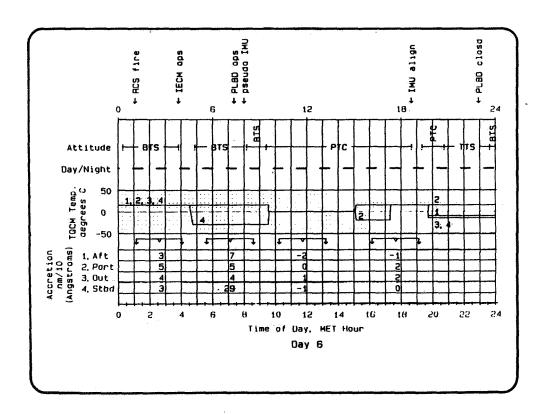
On day 6, the Orbiter left the BTS condition and the TQCM accretions show an immediate response. Towards the end of the day the TQCM's were all set to different temperatures in preparation for deorbit. However, because of landing site conditions, deorbit was delayed for 1 day.
