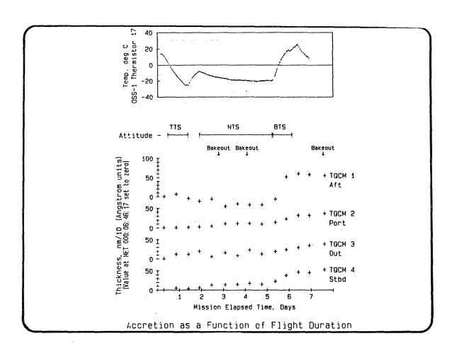
In order to see some of the longer-term trends, the data for the four TQCM's was plotted selecting portions about 10 orbits apart (to simplify the data reduction process). The data shown have been normalized by setting them all to zero at one time (day 0, 06:46:17).
