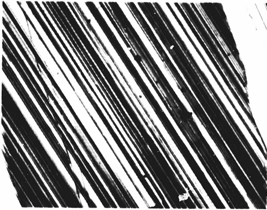
Fig. 2 Region Showing High Twin Density in Semix A-13 (50X)
