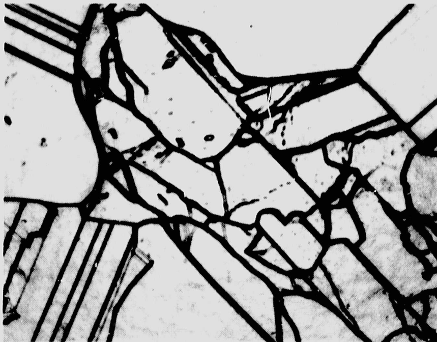
Fig. 9 Many Twin and Grain Boundary Region in Semix D-8 (66X)
