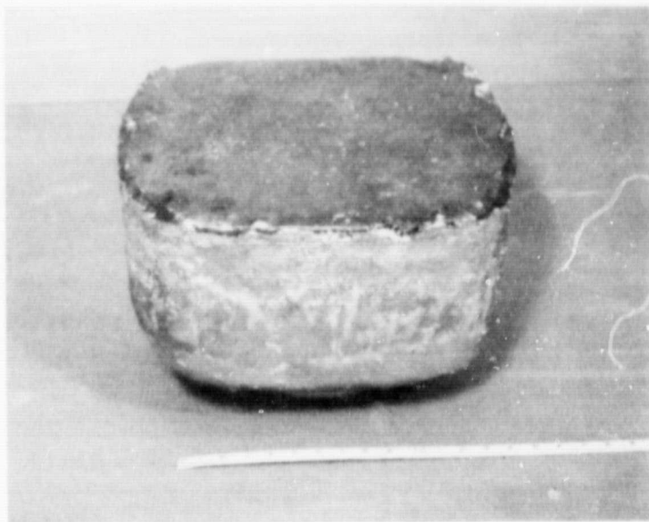
Figure 30. A 5.5 kg, 16 cm x 16 cm cross-section ingot cast in run 353-C using upgraded metallurgical silicon
