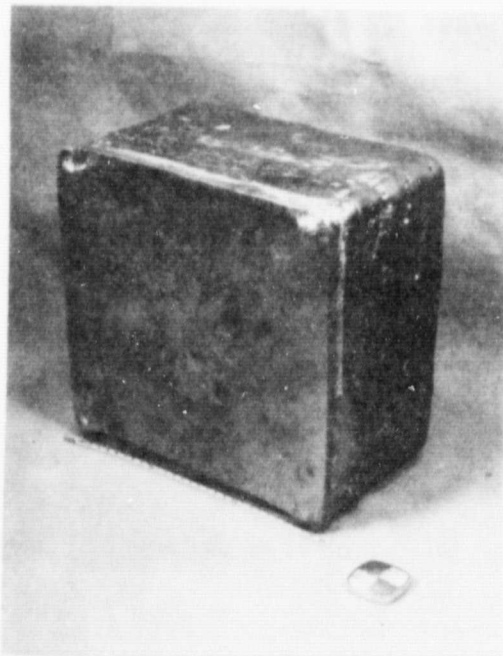
Figure 29. View of an ingot with no problem of broken corners when the crucible edge is not adjacent to the heater
