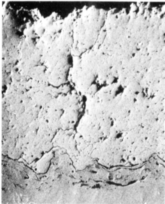
Figure 30 Light Microscope (Top) and SEM (Bottom) Photographs of Pre-Test (Left) and Post-Test (Right) Microstructures of a 12 w/o Y_2O_3 Stabilized ZrO_2 Coating.
