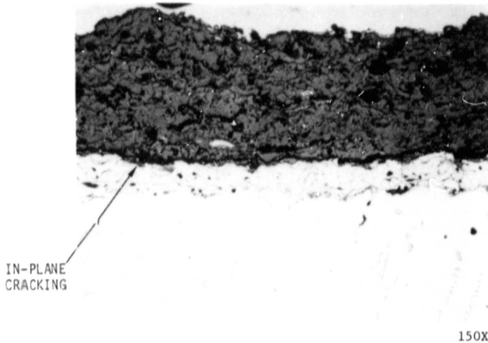
Figure 54 Typical 20 w/o Y_2O_3 Stabilized ZrO_2 Microstructure Observed on First Engine Test Vane. Arrow indicates in-plane cracking.
