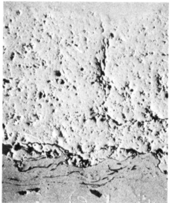
Figure 30 Light Microscope (Top) and SEM (Bottom) Photographs of Pre-Test (Left) and Post-Test (Right) Microstructures of a 12 w/o Y_2O_3 Stabilized ZrO_2 Coating.
