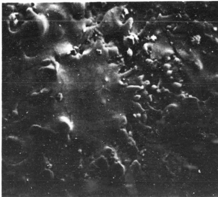
Figure 20. Cross section of specimen wall showing layered particles.
