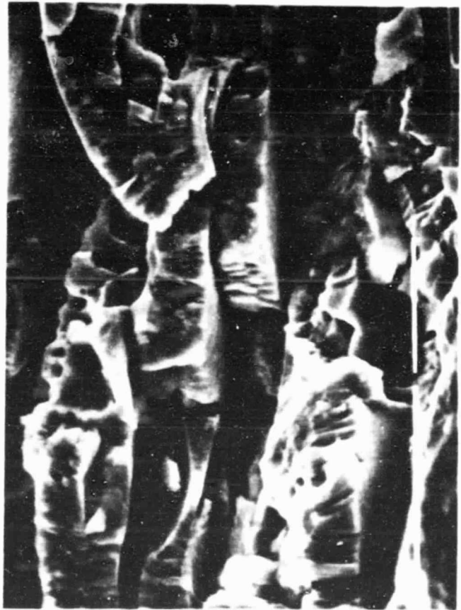
Figure 4. SEM micrographs, low density ZrO_2 sample in fractured cross-section. 390, 1170 and 3900X magnifications. 6.4 micron bar (separated stripe) is shown at the high magnification.
