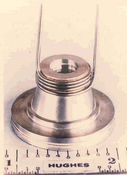
Figure 2-10. A metal pressure seal for a probe pressure vessel is shown with its disassembled testing fixture after undergoing a sealing test in a simulated Venusian descent environment.
