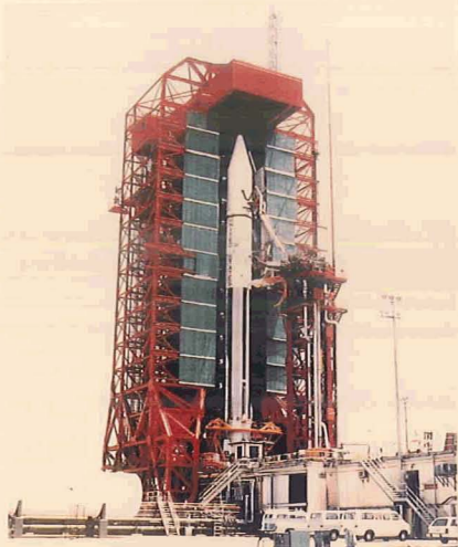
Figure 2-7. An Atlas-Centaur, NASA's standard launcher for payloads of intermediate weight, was used to launch each of the Pioneer Venus spacecraft.
