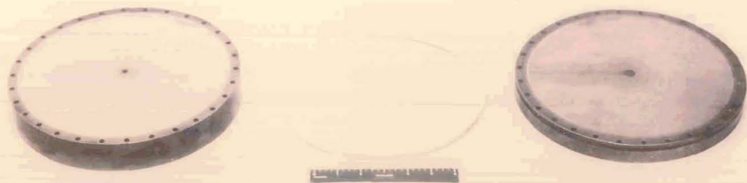
Figure 2-10. A metal pressure seal for a probe pressure vessel is shown with its disassembled testing fixture after undergoing a sealing test in a simulated Venusian descent environment.
