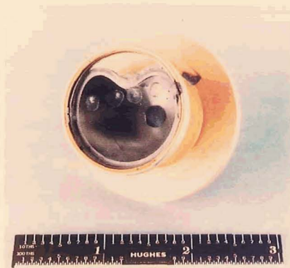
Figure 2-11. (a) Shown is a side view of the 3.175-cm (1.25-in.) diameter sapphire window assembly after a simulated Venusian descent pressure and temperature test. The assembly consists of an inconel housing with a kovar-sheathed heater wrapped around a brazed sapphire window. (b) Shows the result of pressure testing a sapphire window and mount representative of the probe windows. Note that the mount failed prior to the window itself. The test failure pressure was approximately three times the maximum amount expected at the surface of Venus.
