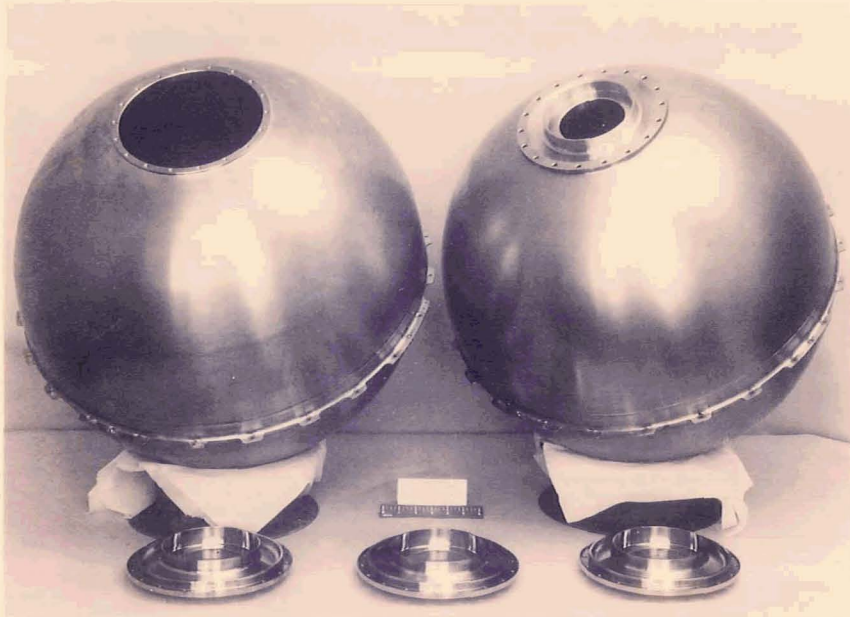
Figure 3-6. A solid propellant rocket motor provided thrust to place the Orbiter into an elliptical orbit around Venus. This orbit insertion motor was supplied by Thiokol Corporation. The picture shows the motor case and the nozzle closure of titanium alloy forgings. The case consisted of two 0.028-inch thick hemispheres joined by a single weld. The nozzle closure, which fastened to the case, was the structural element of the nozzle. Integral bosses allowed attachment of nozzle and igniter, and a scalloped flange was used to attach the motor to the spacecraft.
