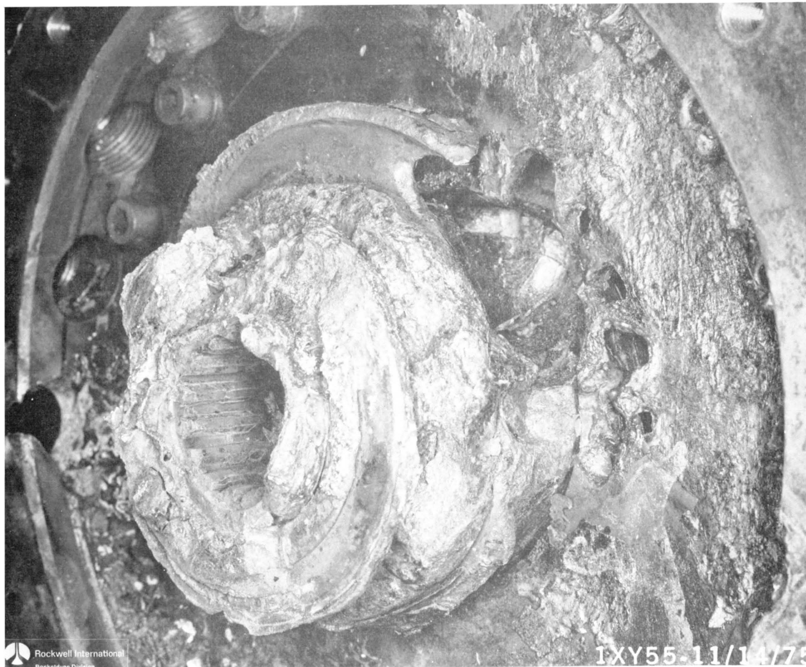
Figure 64. Posttest 222 Fire Showing Outboard Slave Seal Mate Ring, Remaining Helium Seal Mate Ring, and LOX Seal Housing
