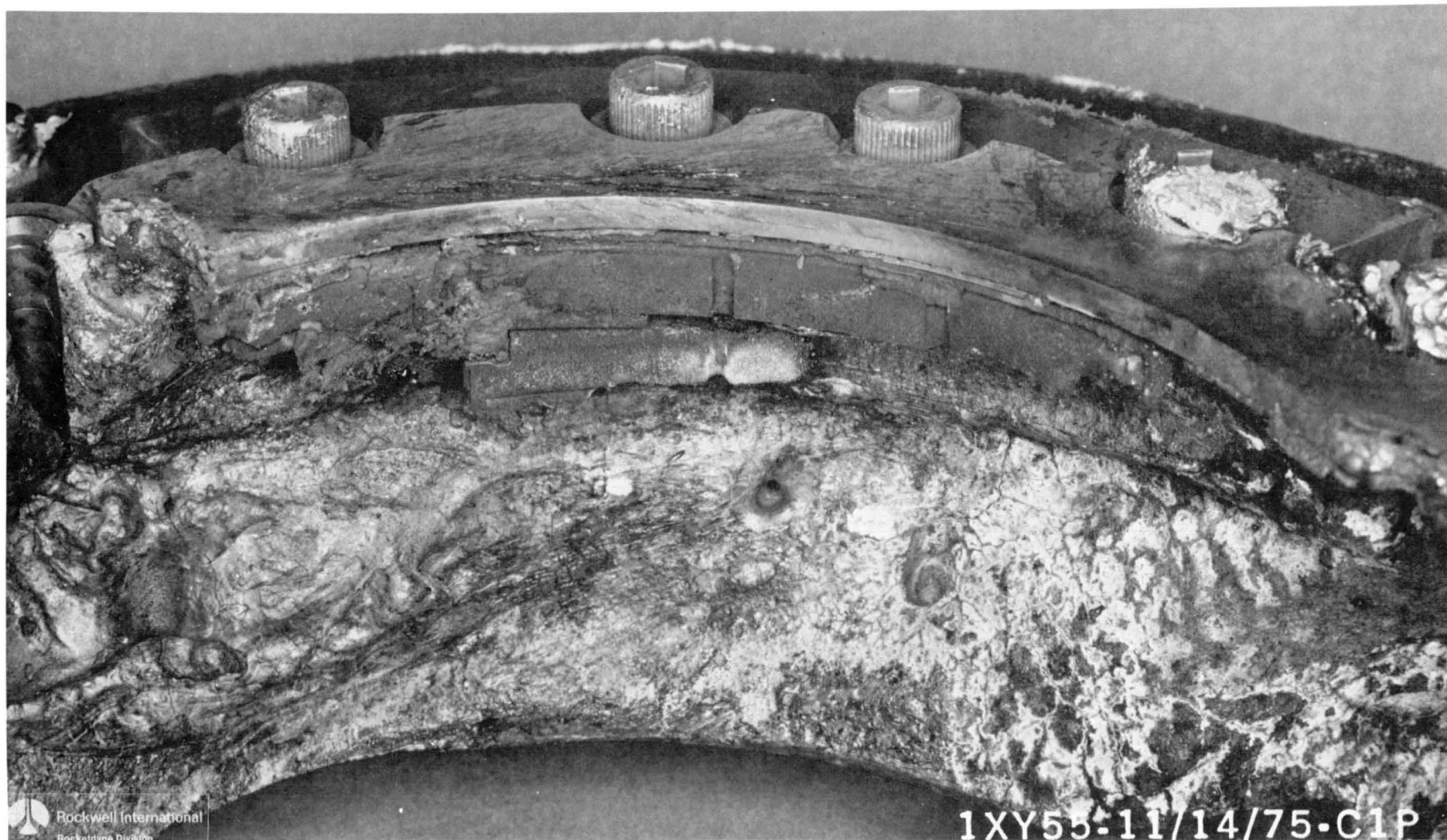
Figure 66. Posttest 222 Fire Showing Helium Seal LOX Side Carbon Segment
