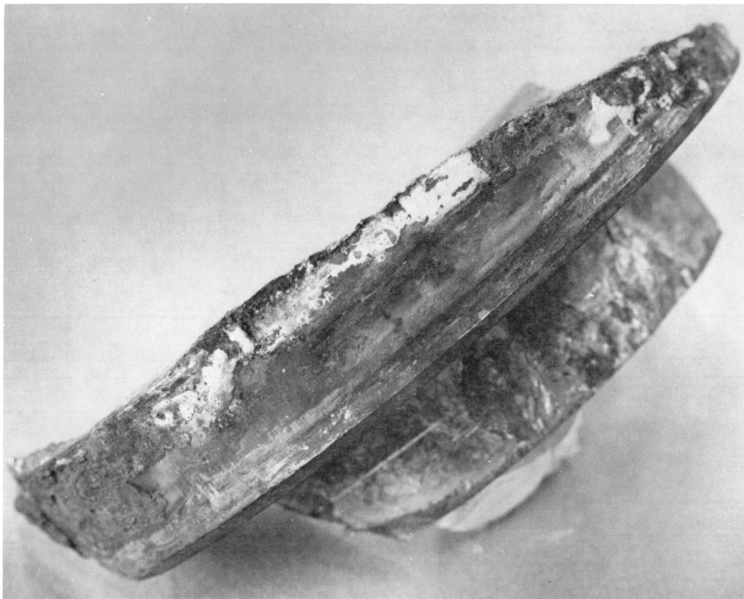
Figure 65. Posttest 222 Fire Showing Helium Seal Mate Ring
