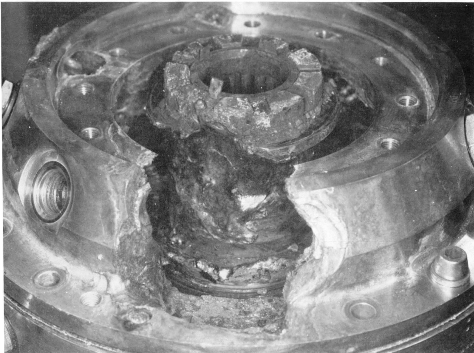
Figure 129. Helium Seal Drain and Outboard Seal Area, Posttest 176
