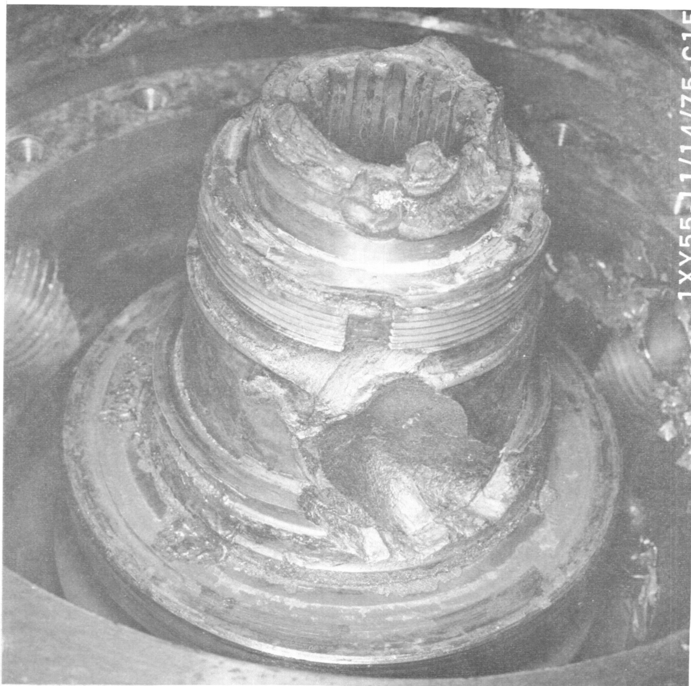
Figure 68. Posttest 222 Showing LOX Seal Mate Ring and Shaft Burning
