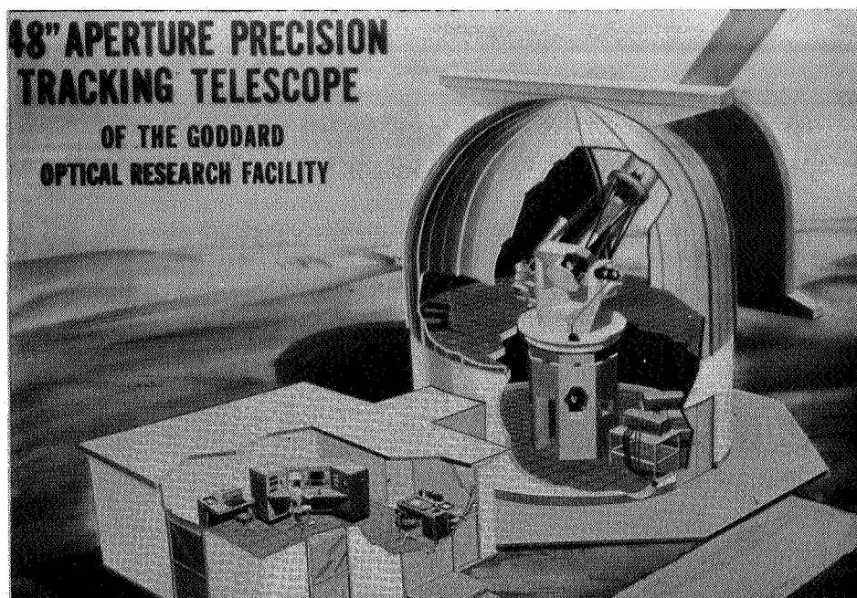
Fig. 12. Transmit/Receive telescope at the GORF.
