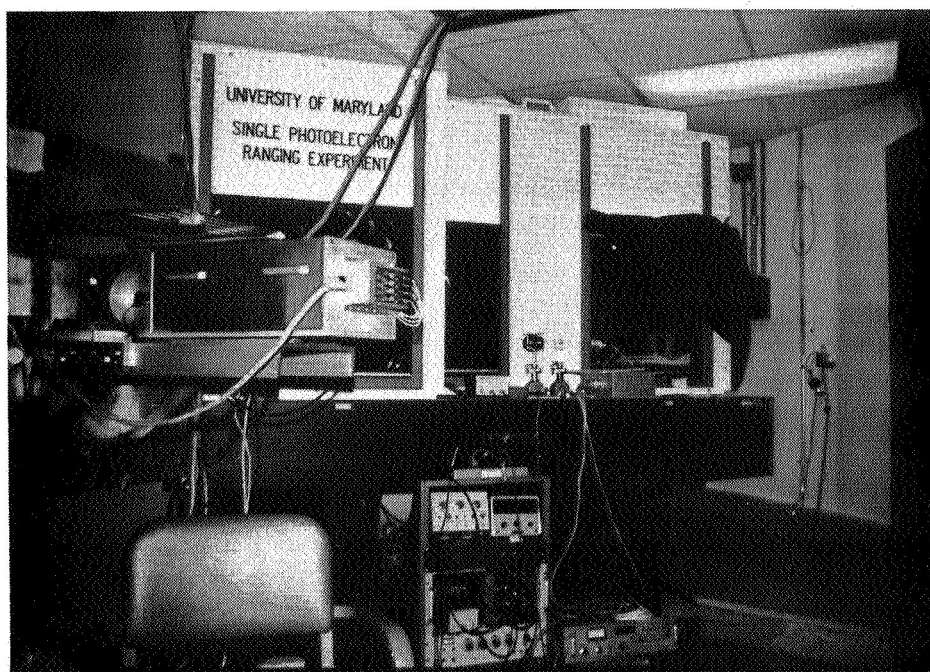
Fig. 13. Optical and electronic equipment for transmitting and receiving laser pulses.
