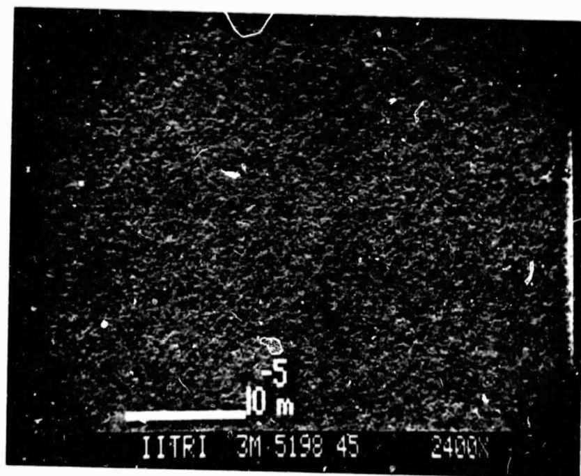
Figure 2.9.5c: 3M 5198 Oxide Surface, 45 Degrees, 2400x
