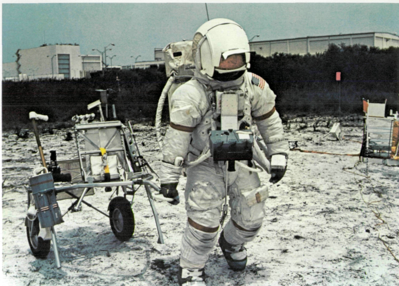
A prototype of the Modular Equipment Transporter (MET) that increases mobility of Apollo 14 astronauts on the lunar surface. MET, called "rickshaw" by its astronaut pullers, is a hand-drawn vehicle that serves as a portable workbench, a camera mount, and as a platform for the Lunar Portable Magnetometer experiment.
