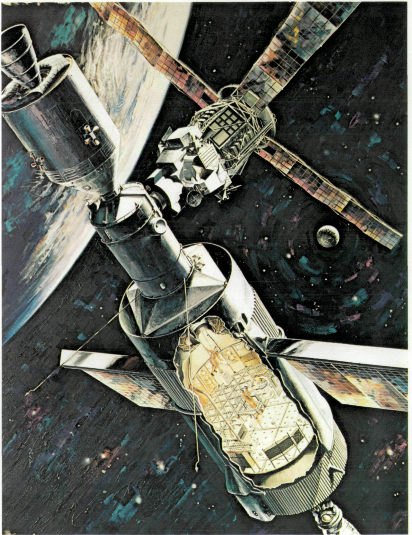
A cutaway view of Skylab in Earth orbit.
