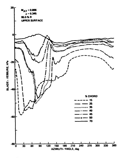
Fig. 14. Model OLS rotor upper-surface ' Source versus azimuth for M<sub>AT</sub> = '.896
