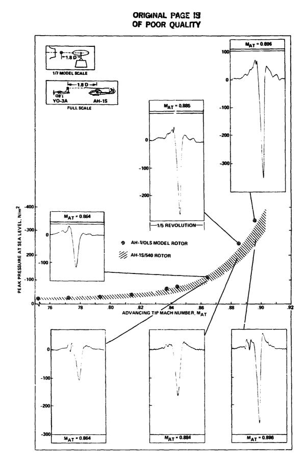
Fig. 8. Comparison of model and full-scale acoustic waveforms for an in-plane microphone 1.8 rotor diameters ahead.
