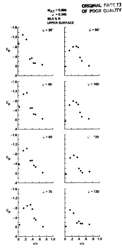
Fig. 15. Model OLS rotor upper-surface chordwise pressure coefficient versus azimuth for  $M_{AT} = 0.896$ , 95.5% R.
