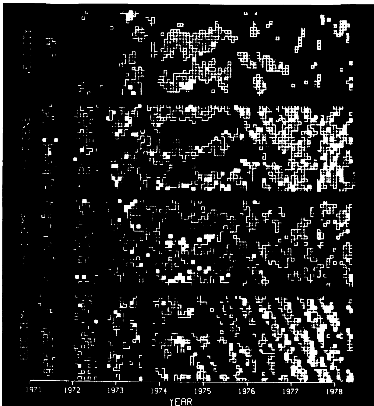
Figure 1. Daily averages of solar wind proton bulk speed, density, and temperature and electron temperature arranged in sequential strips of 27-day Carrington rotations, with values increasing from dark to light shades, after Feldman et al. (1979). (See their colored version and code table for quantitative information.)
