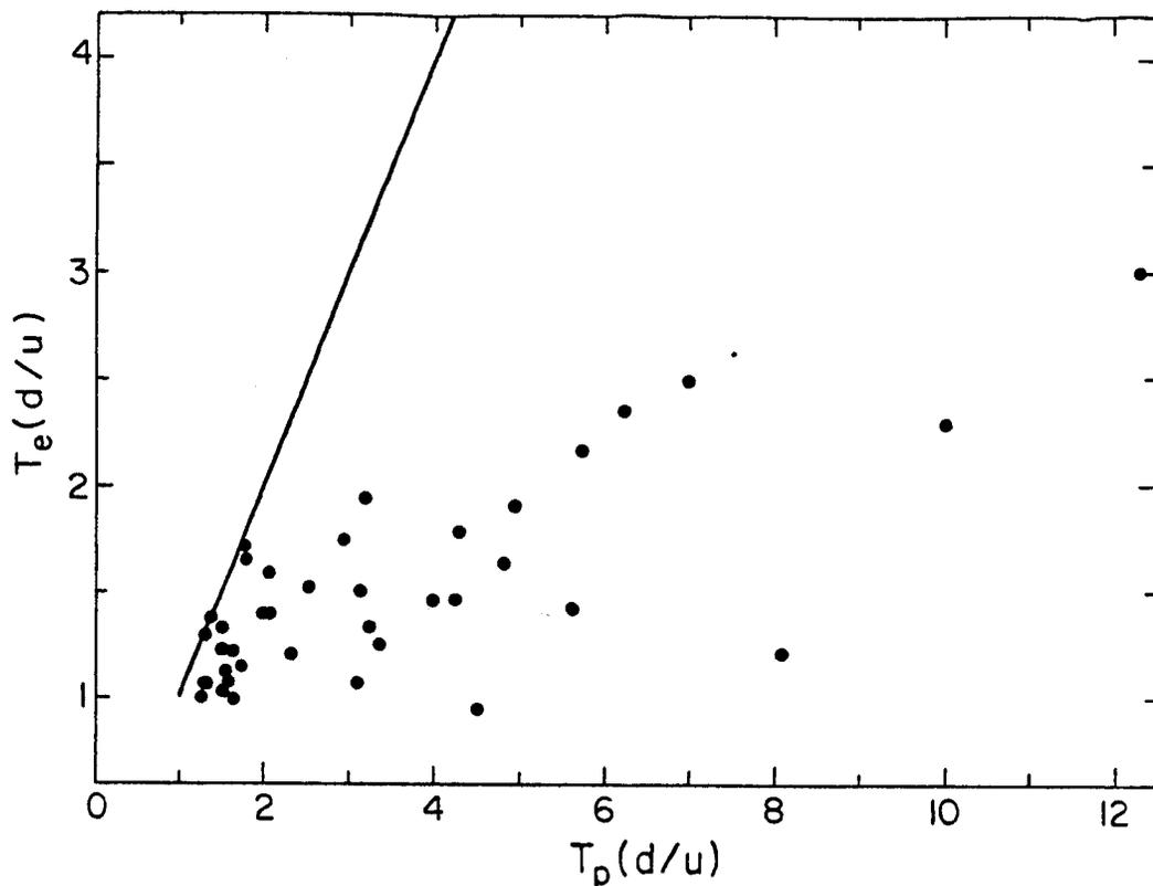
Figure 2. A scatter plot showing the correlation between the ratios of downstream to upstream electron and proton temperatures at 41 forward interplanetary shocks observed at ISEE 3 between August 1978 and December 1979. The solid line represents equal ratios of downstream to upstream electron and proton temperatures.
