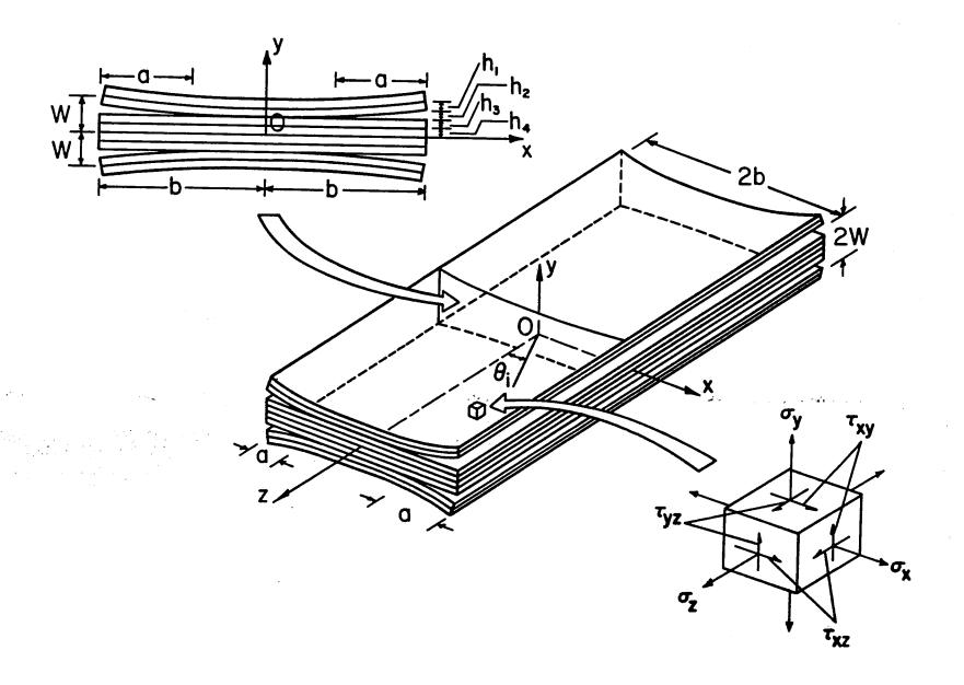
Fig. 1 Delaminations in a  $[\theta_1/\theta_2/\theta_3/.../\theta_3/\theta_2/\theta_1]$  Fiber-Reinforced Composite Laminate.
