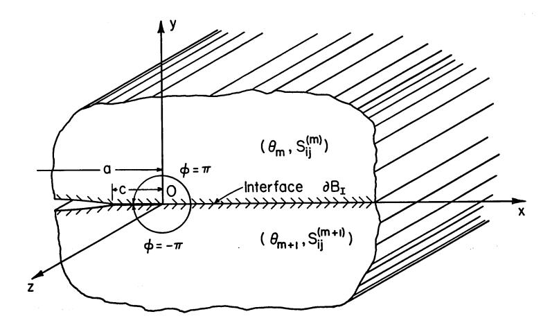
Fig. 3 Coordinates and Geometry of a Delamination with Finite Length of Crack-Surface Closure between  $\theta_m$  and  $\theta_{m+1}$  Plies.
