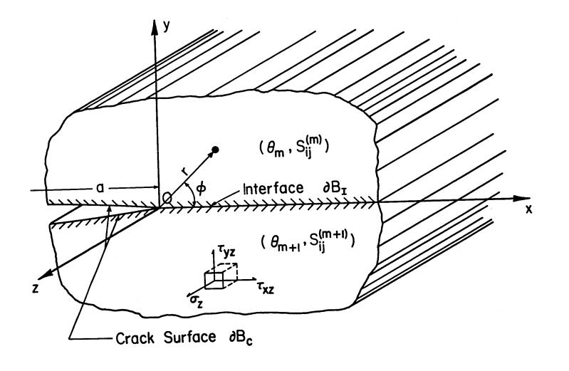
Fig. 2 Coordinates and Geometry of a Delamination with Open Crack Surfaces between  $\theta_m$  and  $\theta_{m+1}$  Plies.
