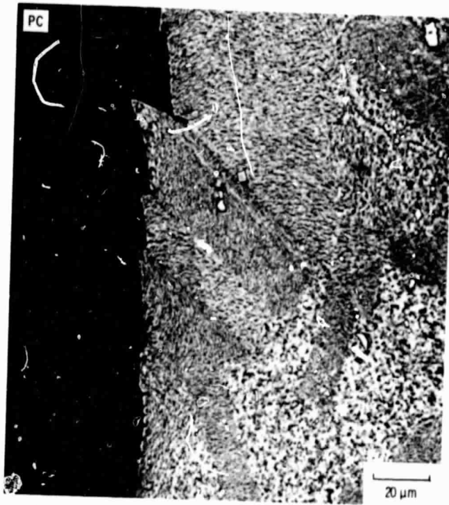
Figure 11. - Tongue on Udimet 700 at 1400°F in PC type of loading.
