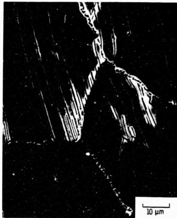
Figure 16. - Examples of CP cracking in 316 S.S. at 1300°F.
