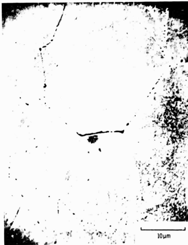
Figure 17. - Example of CP cracking in Tantalum alloy T-111 in high vacuum.
