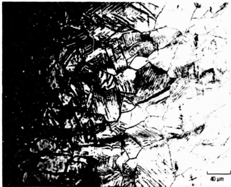
Figure 6. - Example of CC cracking 316 SS, 1300°F, 50% N_F .
