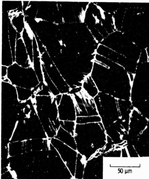
Figure 16. - Examples of CP cracking in 316 S.S. at 1300°F.
