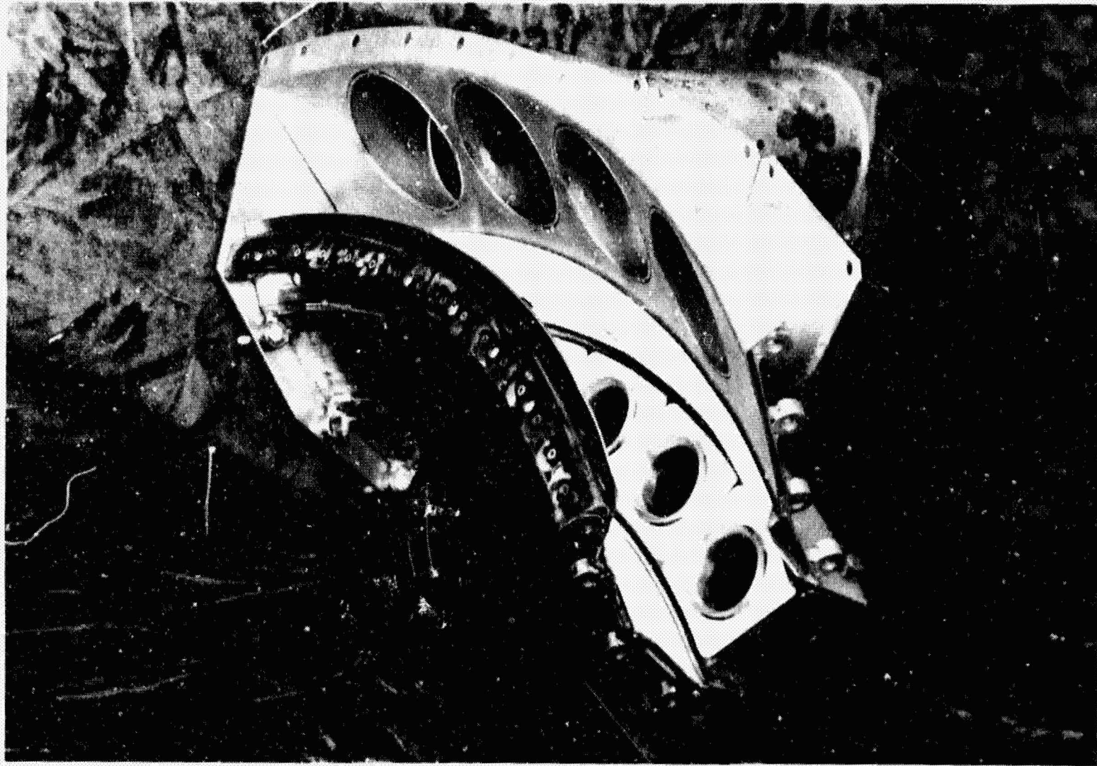
Figure 9. Reverse-Flow Sector-Combustor Assembly Showing Juncture of Main Stage Exit with the Pilot Stage.
