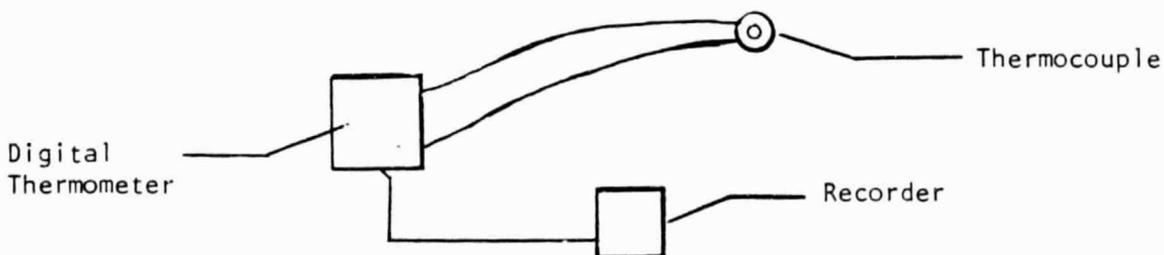
Figure C-23 - Schematic of the Temp. Sensing System
