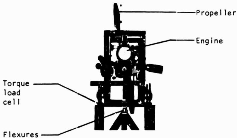
Figure 2.6 - Torque System
