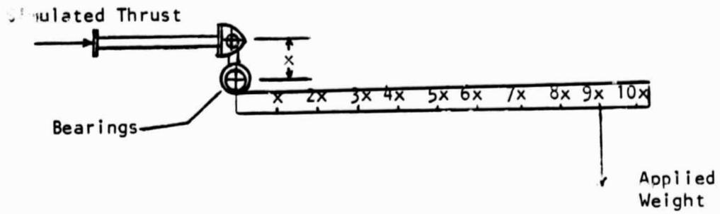
Figure C-9 - Schematic of the Thrust Calibration Stand
