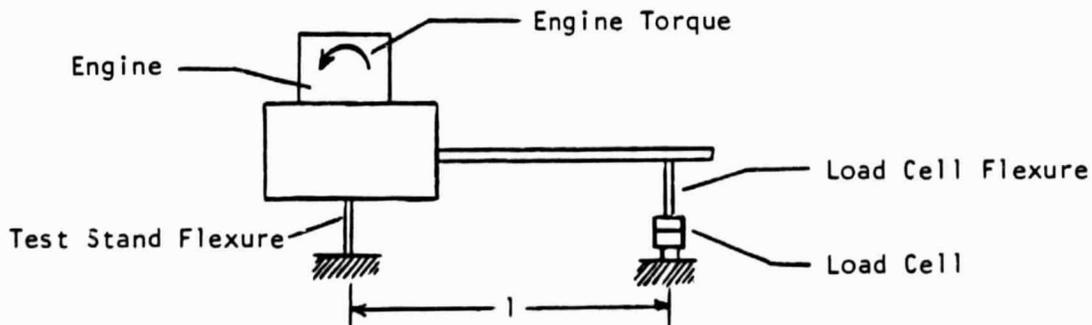
Figure C1 - Schematic for Obtaining Torque
