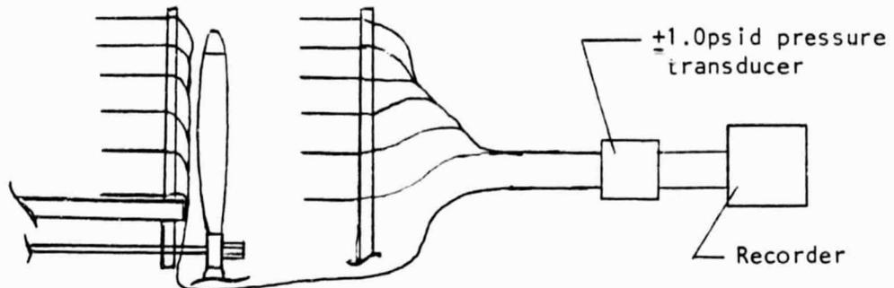
Figure C-18 - Rake Placement to obtain  $\Delta P$
