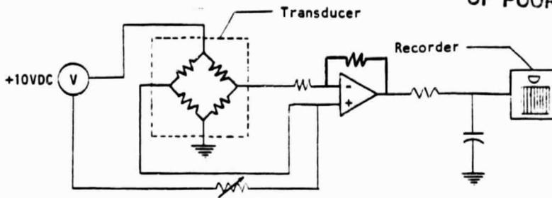
Figure C-8 - Amplification Circuit Diagram
