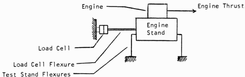
Figure C-7 - Schematic of the method for obtaining thrust
