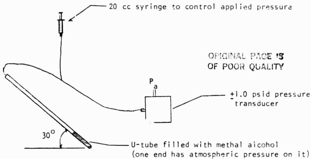
Figure C-21 - Schematic of the  $\Delta P$  Calibration Device
