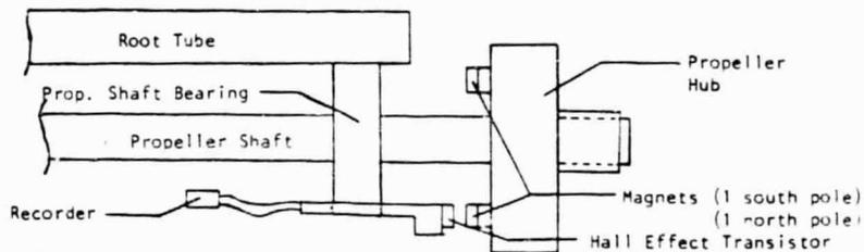
Figure C-1 - Positioning of the Hall Effect Transistor
