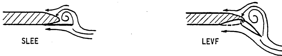
Fig. 1.4 Schematic mechanism of leading-edge flows over a wing with SLEE and LEVF. (Streamwise cut)
