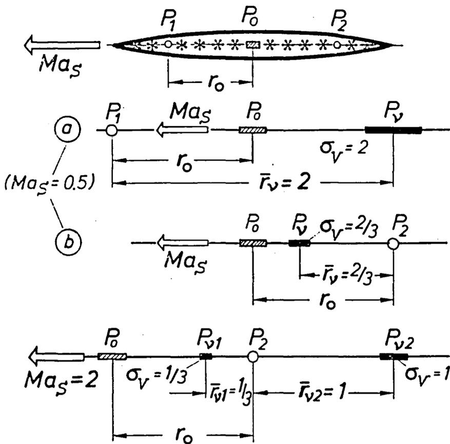
Fig. 13: Radiation Processes of Moving Source Elements in Field Points on the Orbit and the Physical Phenomena, Leading to the Exact Cancellation of the Effect of Mach Number in the Field Quantities ( $\bar{r}_v = r_v / r_o = \sigma_v$ ).
