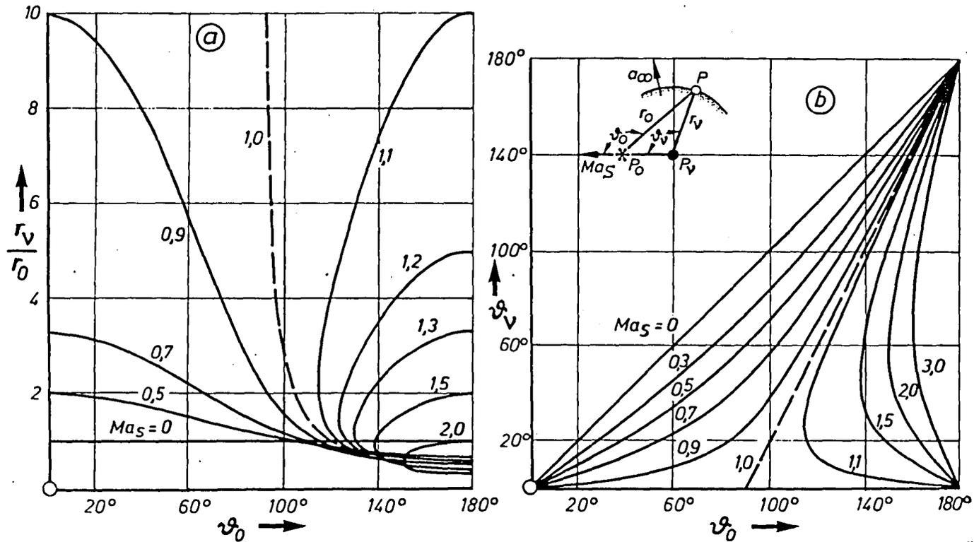
Fig. 3: Universal Relationships for Determination of Radiation Quantities  $r_v$  and  $\theta_v$  of Disturbance Signals, Hitting a Moving Disturbance Source at Varying Mach Numbers  $Ma_S$  at the Field Points  $P(r_0, \theta_0)$  at Time  $t_0$ .
