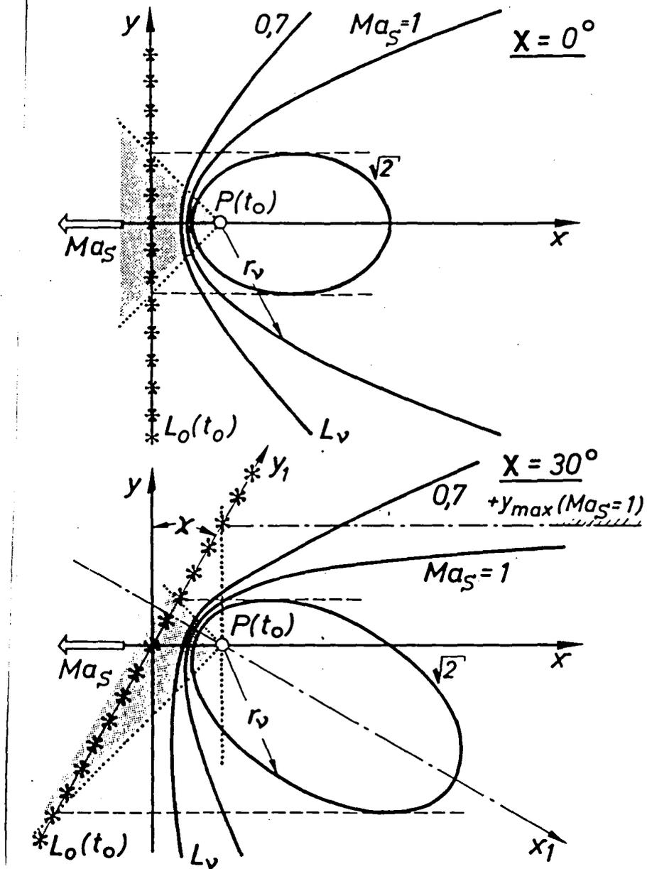
Fig. 11: Radiation Processes of Moving Source Lines of Infinite Length with Various Mach Numbers and Various Orientations to the Path Line with the Disturbance Signals from the  $L_v$  lines Reaching the Field Point  $P(x,0,0)$  Simultaneously at time  $t_0$ .
