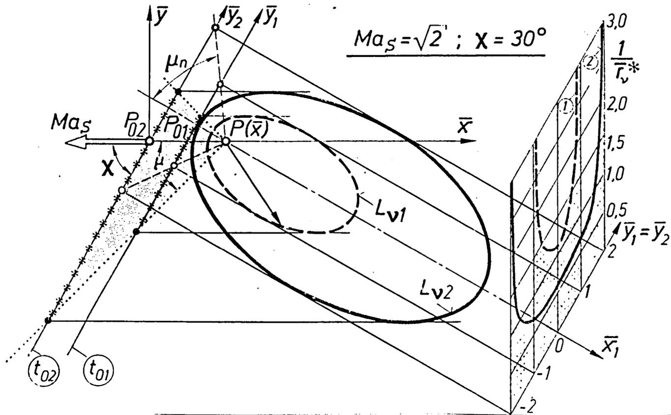
Fig. 12: Radiation Processes from a Moving Source Line in the Case of Supersonic Mach Numbers and Correlated Emission Lines  $L_{v1}$  and  $L_{v2}$  with Disturbance Signals reaching Field Point  $P$  at Times  $t_{01}$  and  $t_{02}$  and always producing Constant Field Quantities for  $\bar{x} > x_0$ .
