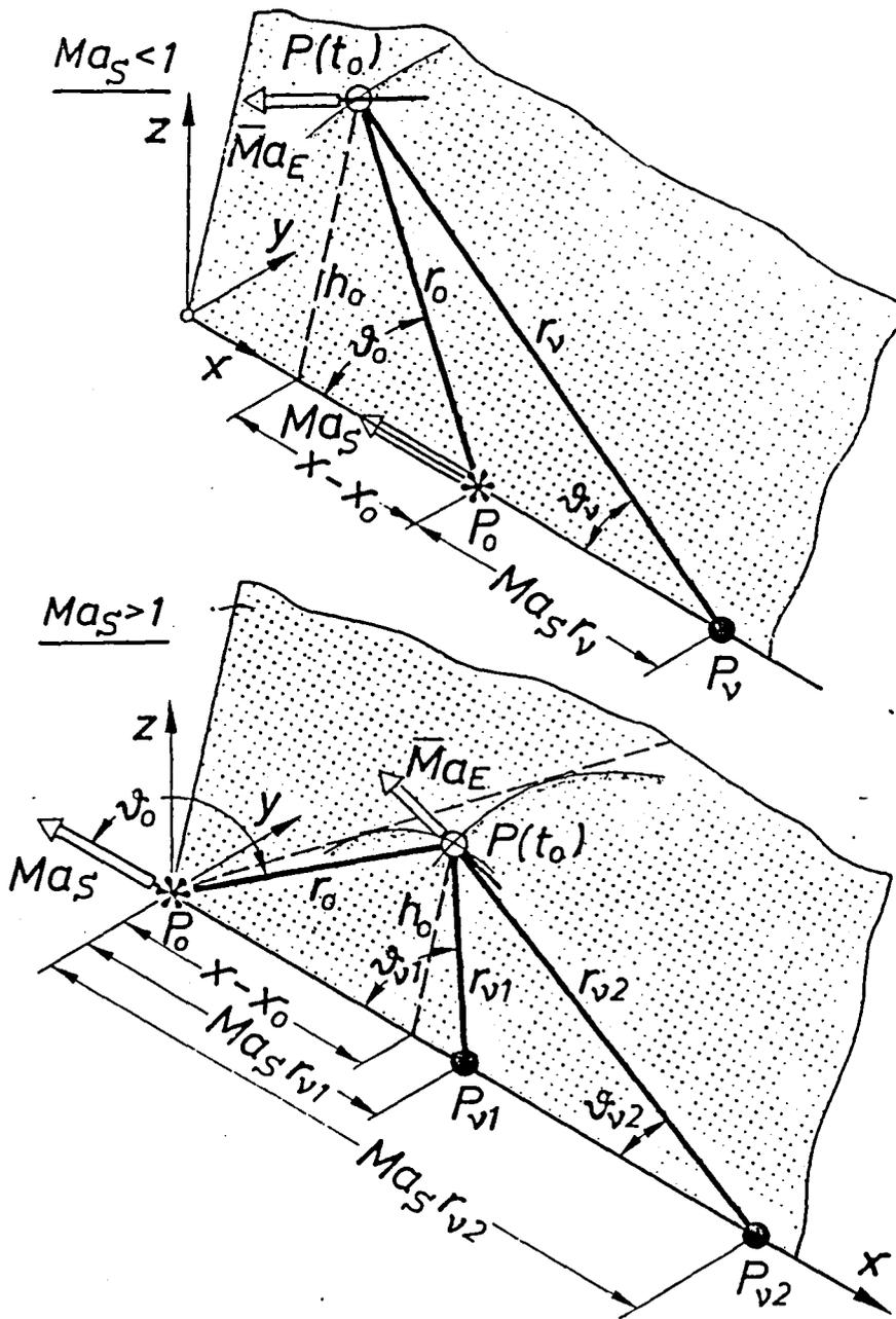
Fig. 2: Kinematic Relationships in the Disturbance Propagation of Moving Disturbance Sources in a Homogeneous Medium at Rest with Infinite Dimensions.
