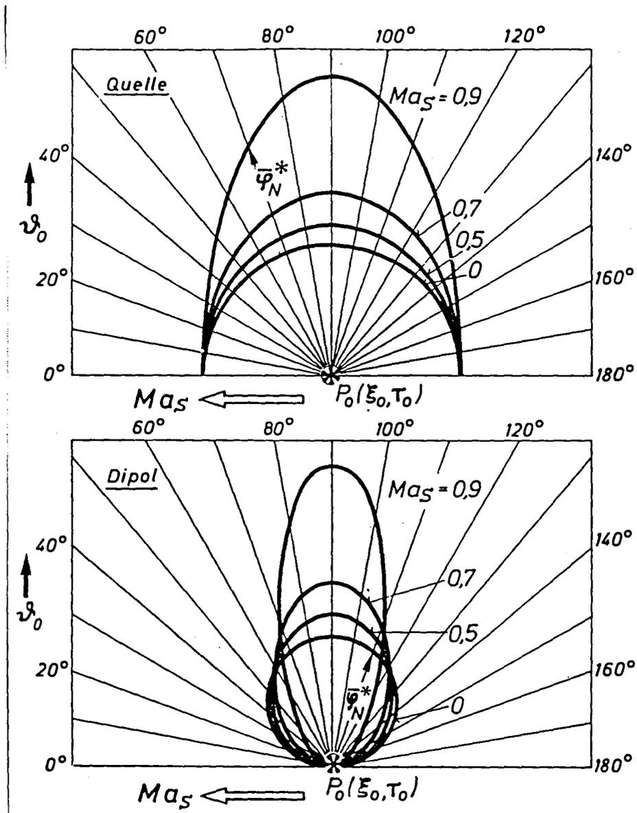
Fig. 15: Near Field Portions of the Disturbance Potential on a Unit Sphere with  $r_0 = 1$  around  $\xi_0$  with Various Mach Numbers of a Moving Source and a Moving Dipole.
