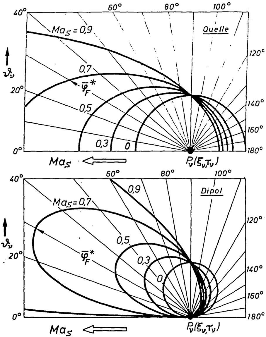
Fig. 16: Distant Field Portion of the Disturbance Potential in the Disturbance Waves with  $\bar{r}_v = 1$  around  $\xi_v$  at Various Mach Numbers of a Moving Source and a Moving Dipole.
