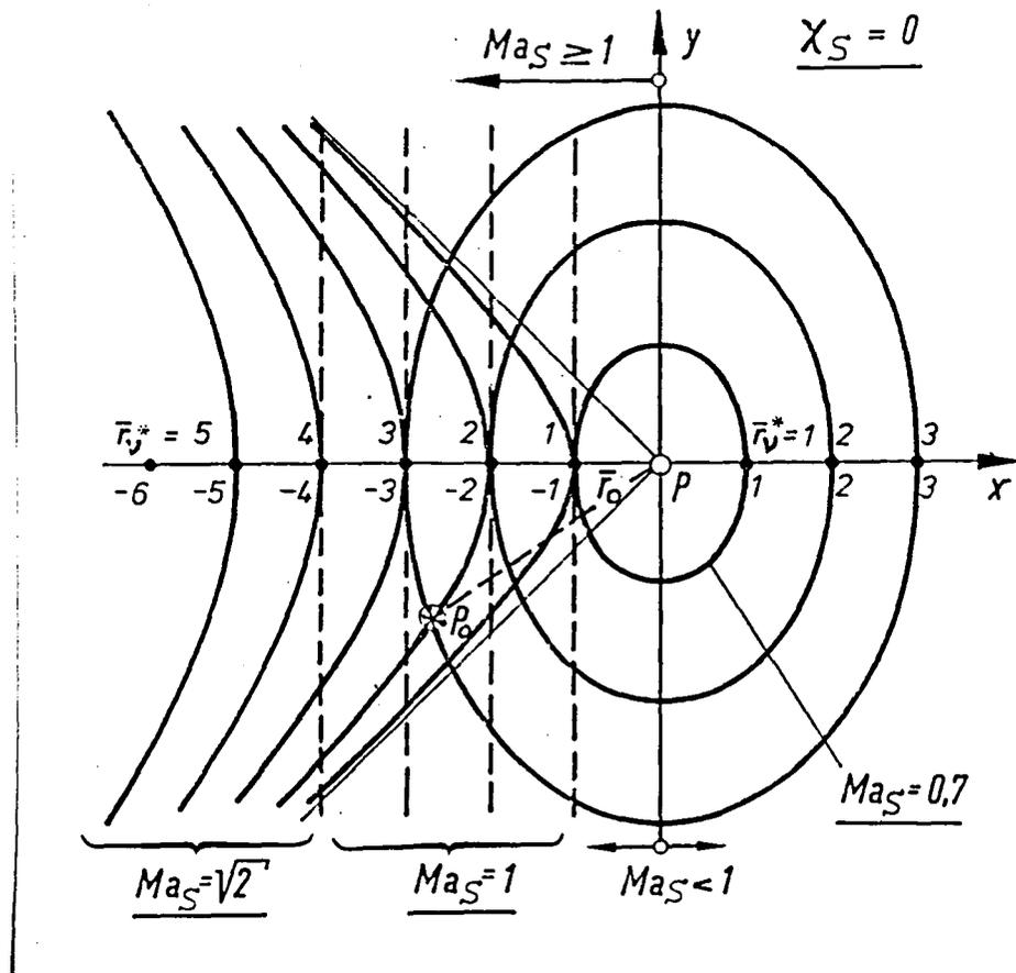
Fig. 14: Surfaces in Space with Constant Values of  $r_v^*$  at Subsonic, Sonic and Supersonic Velocities of the Disturbance Sources with the Axis  $x$  of Symmetry Through the Field Point  $P$ .
