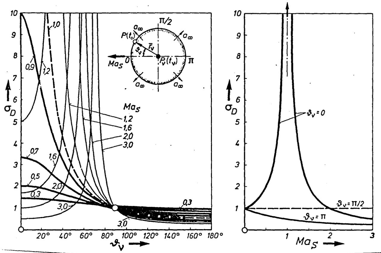
Fig. 8: The Doppler Factor  $\sigma_D$  in the Propagation of Spherically Symmetrical Waves from Moving Disturbance Sources in a Homogeneous Medium at Rest.
