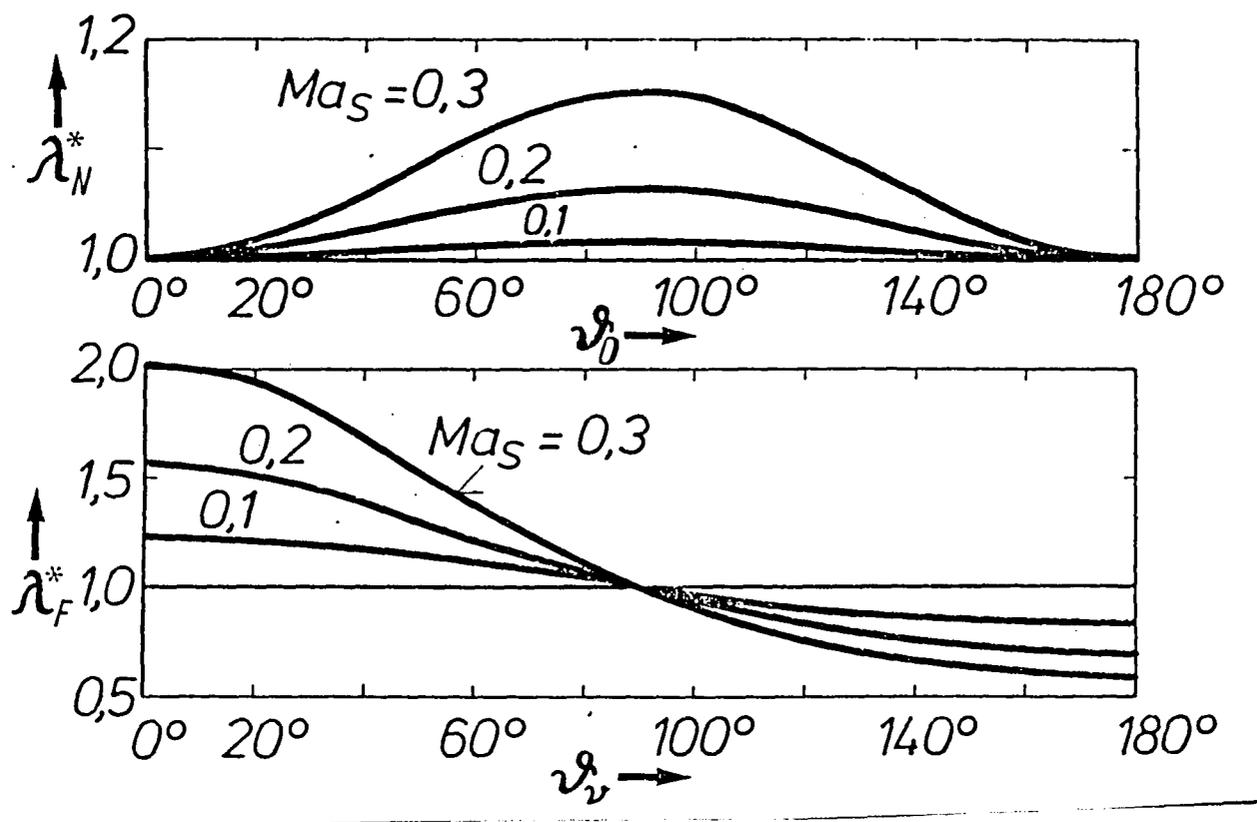
Fig. 18: The Ratio of the Nonsteady to the Quasi-Steady Field Quantities in the Near Field and Distant Field Portions of a Moving Source
