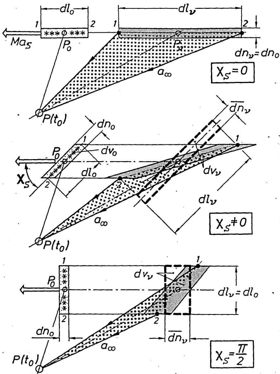
Fig. 5: Production of the Spatial Correlation Functions  $\sigma_V$  as a Result of the Actual Volume Expansion of the Emission Elements in the Case of Various Orientations of the Disturbance source in Space or to the Path Line ( $\sigma_V = \sigma_L \sigma_N$ ).
