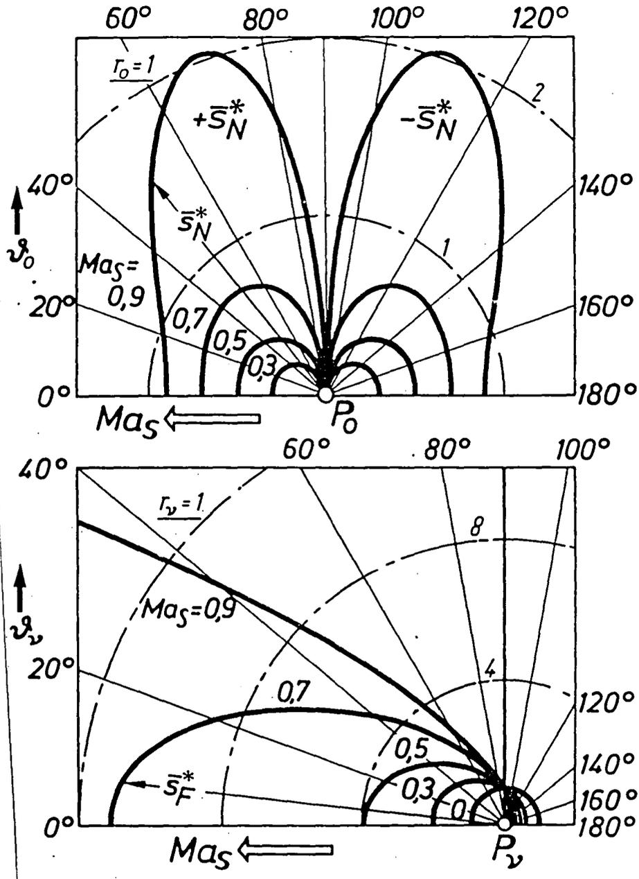
Fig. 17: Near Field and Distant Field Portions of the Disturbance Quantities on a Unit Sphere with  $\bar{r}_0 = 1$  around  $\xi_0$  or with  $\bar{r}_v = 1$  around  $\xi$  with Various Mach Numbers of a Moving Source. ( $s_N^* = s_N / \omega_v \bar{S}$  or  $s_F^* = s_F / \omega_v^2 \bar{D} \cos \psi$ ).
