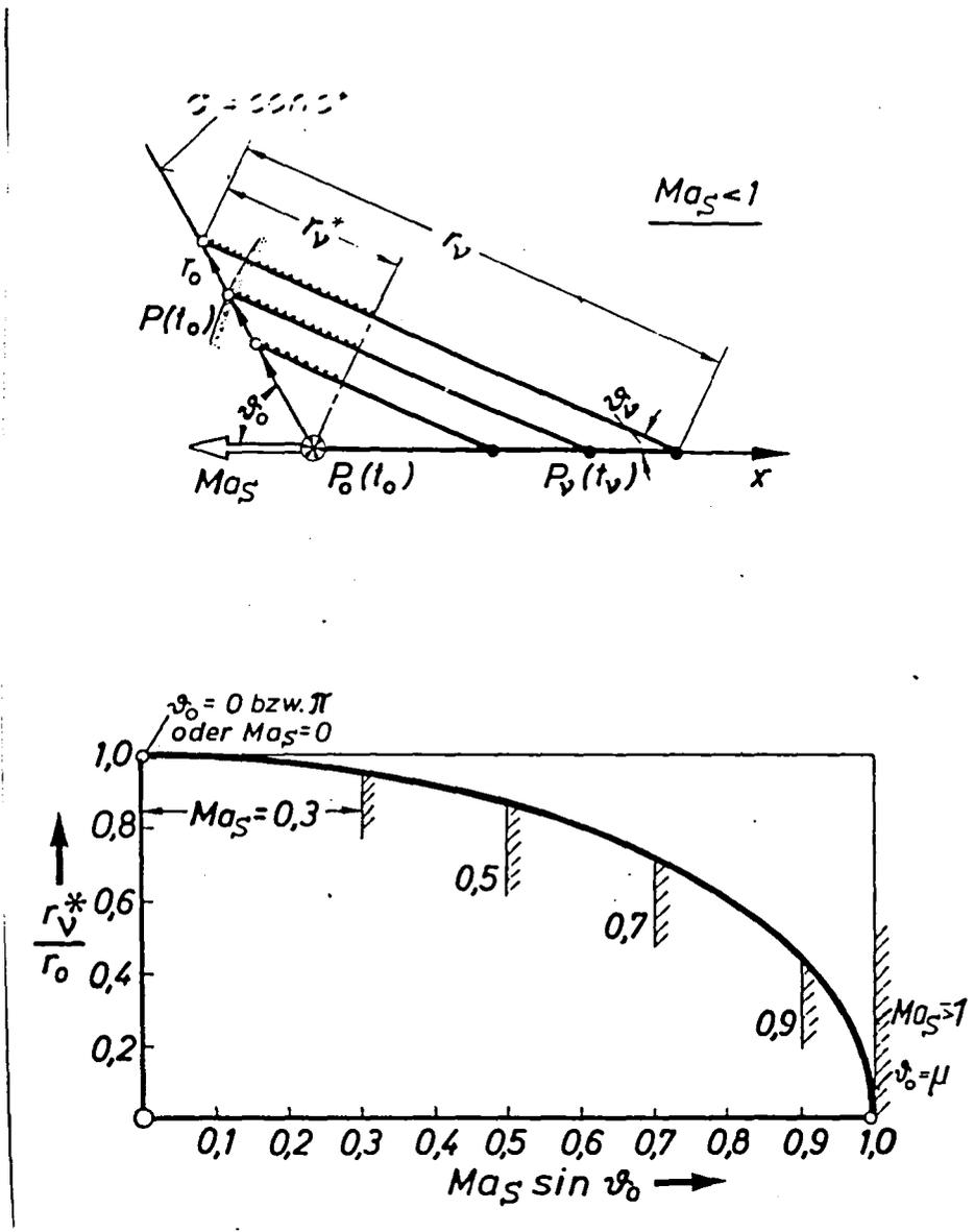
Fig. 10: Universal Representation of the Actual Emission Radii  $r_v^*/r_0$  for Random Field Points in Space with Subsonic and Supersonic Mach Numbers of the Disturbance Sources.
