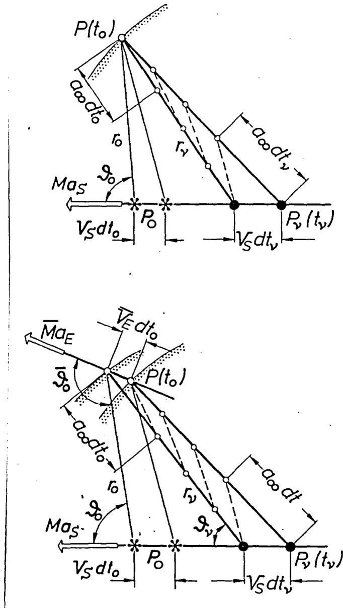
Fig. 7: Production of the Doppler Factor  $\sigma_D$  and  $\sigma_D^*$  as a Result of the Change in Wave Passage Duration  $dt_0$  through a resting or moving Field Point in Comparison to Duration  $dt_v$  of the Emission of Disturbance Signals. ( $\sigma_D, \sigma_D^* = dt_v / dt_0$ ).
