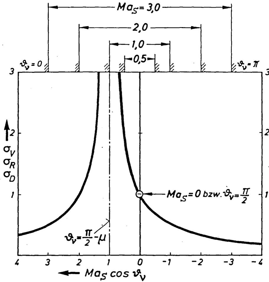
Fig. 9: A Universal Representation of the Correlation Functions  $\sigma_V$ ,  $\sigma_R$  and  $\sigma_D$  in the Propagation of Spherically Symmetrical Disturbance Waves from Moving Singularities.
