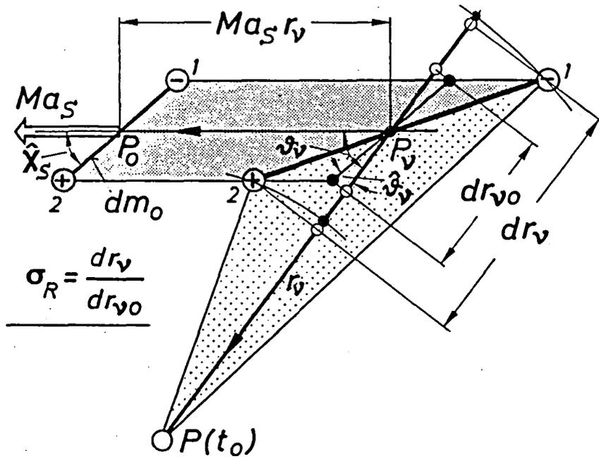
Fig. 6: Production of the Spatial Correlation Function  $\sigma_R$  as a Result of the Actual Shift in Emission Points of Moving Source-Sink Elements of a Dipole, with the Disturbance Signals Reaching Field Point P Simultaneously at Time  $t_0$  ( $\sigma_R = dr_V/dr_{V0}$ ).
