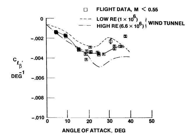
The F-14 data in this figure show the sensitivity with which we can determine stability and control derivatives. Rolling-moment coefficient as a result of differential spoiler deflection ( $C_{\ell\delta}$ ) is shown as a function of angle of attack. It is
