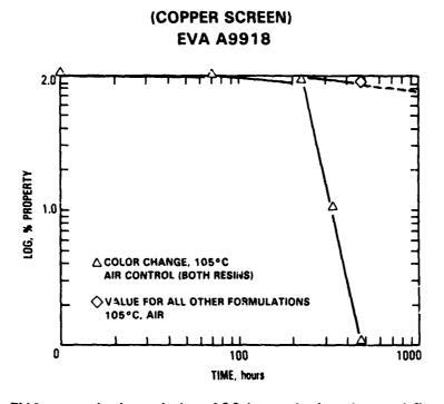
• EVA controls degraded at 400 hours (coloration and flow of resin away from copper screen)
