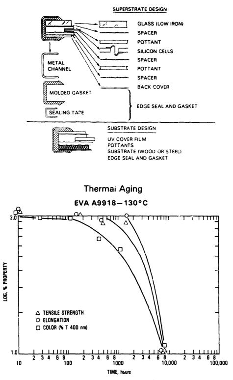
• No change in optical, mechanical, or electrical properties after: 90°C: 7200 hours 105°C: 1000 hours
