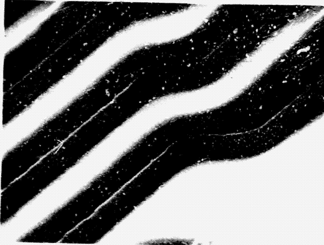
Figure 1. RIE Pattern in 1.2-Micron Al and 2000 Å Over SiO 2 (Photo Resist in Place)
