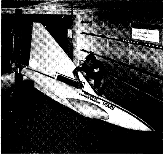
Figure 58. One-third-scale, powered ejector model of the E7 configuration in the Lewis 9- by 15-Foot Wind Tunnel.
