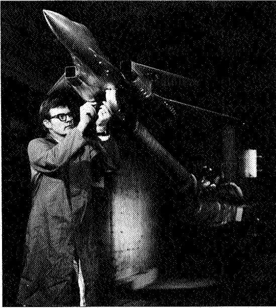
Figure 42. CMAPS model in Ames 11-Foot Wind Tunnel.
