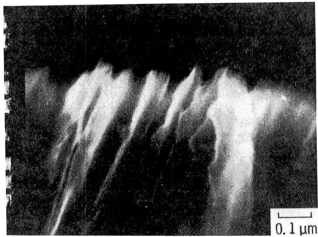
(c) Cross-sectional structure of sputtered MoS 2 film on glass.
