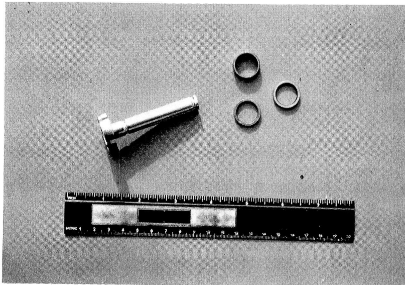
Figure 12 - Ball bearing components ion plated with lead.
