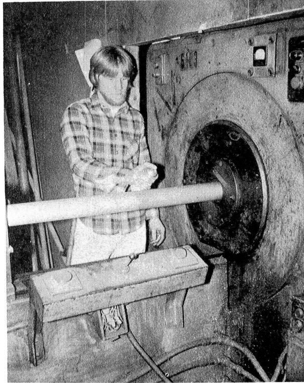
Figure 5 - Aluminum tube coated with an alkyd bonded MoS 2 film.
