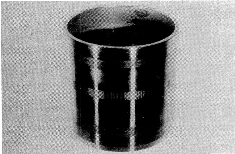
FIGURE 5: Corrosion on Roller Bearing Inner Race
