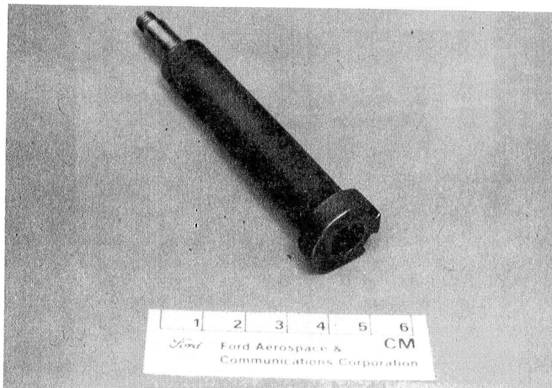
Figure 4 - Power nut coated with a polyimide bonded MoS 2 film.
