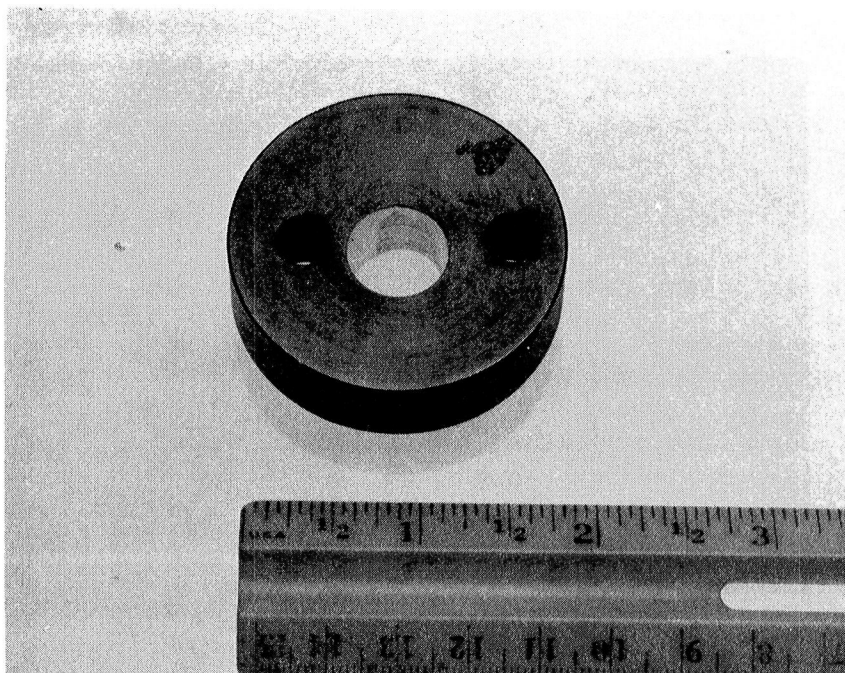
Figure 10 - Cam co-sputtered with \text{MoS}_2 and nickel.
