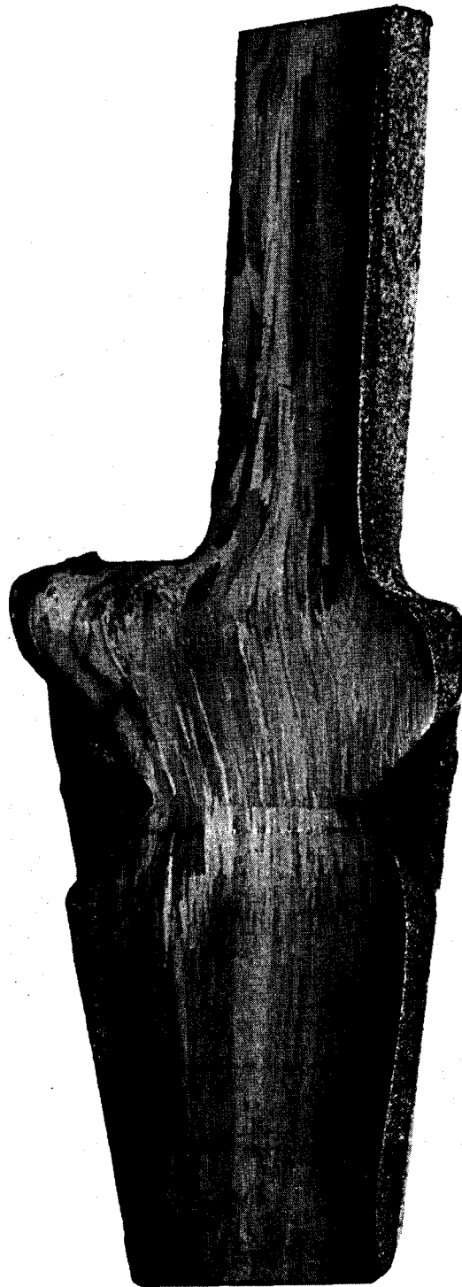
Figure 27. Grain Structure of Forging 15 after Zone Annealing in the Root-to-Airfoil Direction. 2X
