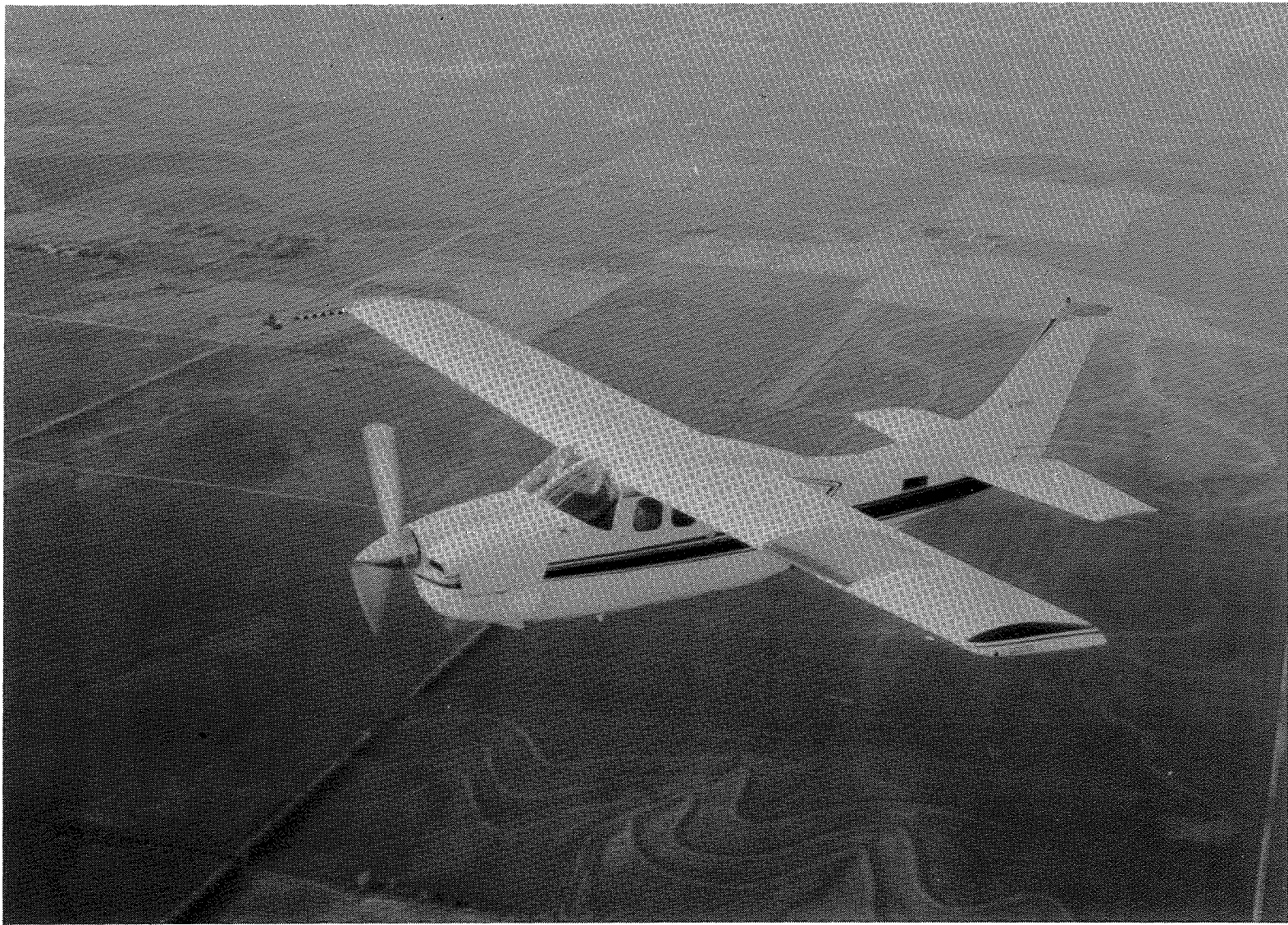
Figure 10.- Cessna P-210 Centurion used in natural laminar flow flight experiments.
